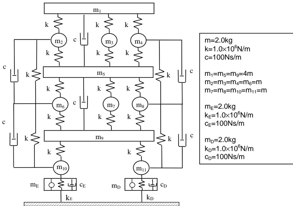
**Figure 1.** Characteristics of the 11 d.o.f. test-system
