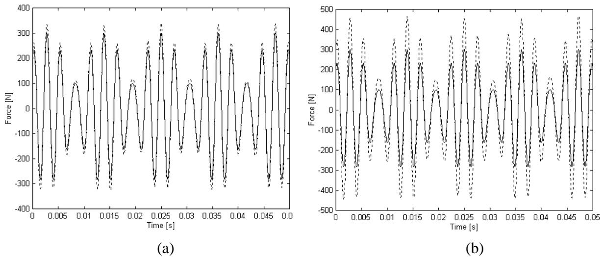
**Figure 4.** Exact (solid line) and reconstructed (dotted line) input forces.
