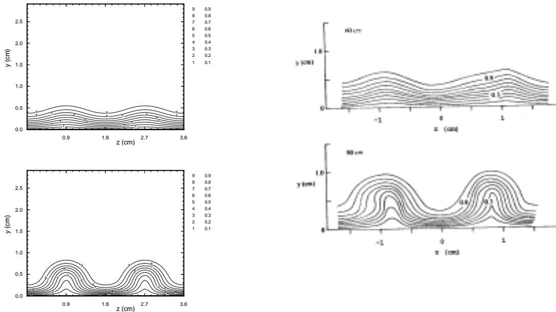
Figure 7: Nonlinear evolution of Görtler vortices. Comparison between PSE results (left) and experimental results (right) (Swearingen and Blackwelder, 1987) for the streamwise velocity distribution in the spanwise plane.
