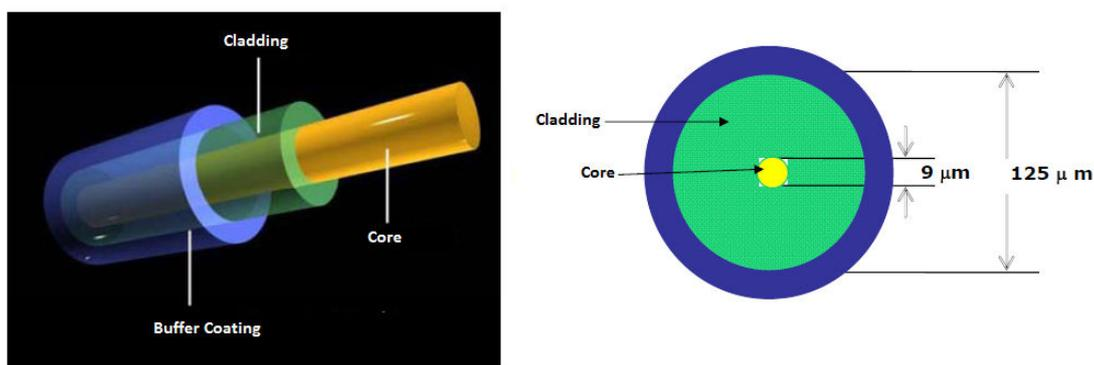
Figure 8 – Structural configuration of a monomode optical fiber. (Classroom notes, 2013)
