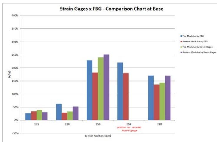
Figure 15 – Strain comparison between Strain Gage and FBG techniques base position.
