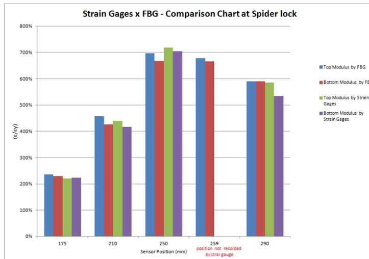
Figure 14 – Strain comparison between Strain Gage and FBG techniques at back position.
