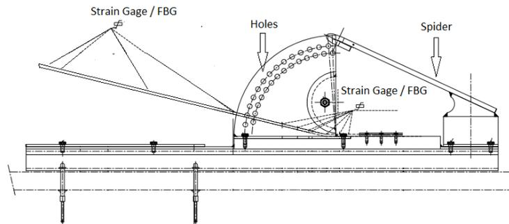
Figure 1 – Curvature device sketch. (Lopes, 2013)
