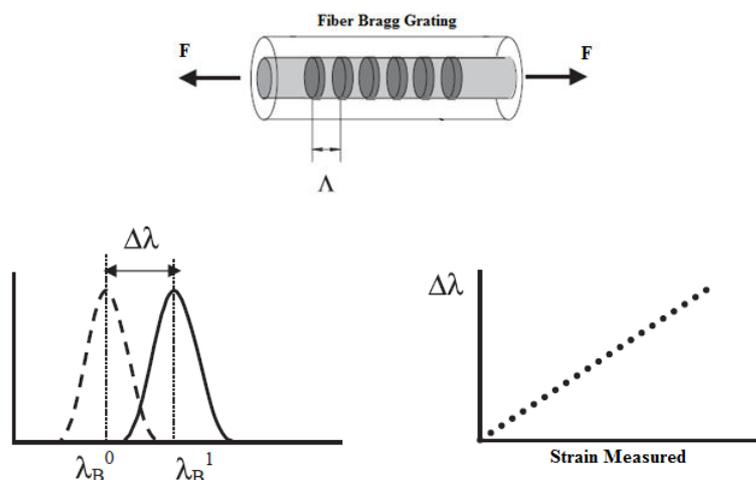
Figure 10 – Relation between applied tension, reflected wavelength variation and strain. (Quintero, 2005)
