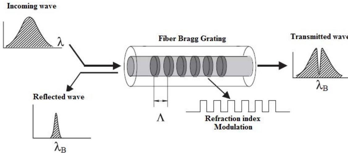
Figure 9 - Sensor operation principle based on the Bragg grating technique. (Quintero, 2005)
