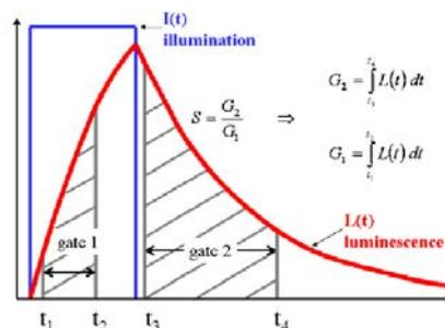
Figure 3. Schematic representation of Life-time method working principle (extracted from Vardaki *et al.* (2010)).
