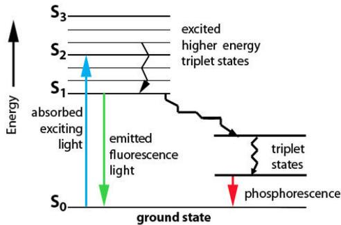
Figure 1. Jablonski diagram and the process of luminescence deactivation.
