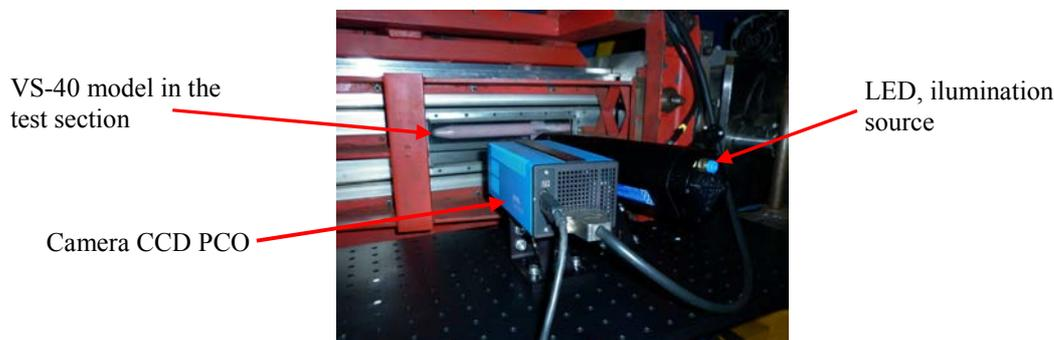
Figure 9. The VS-40 model installed in the TTP test section, the CCD Camera and the illumination device.
