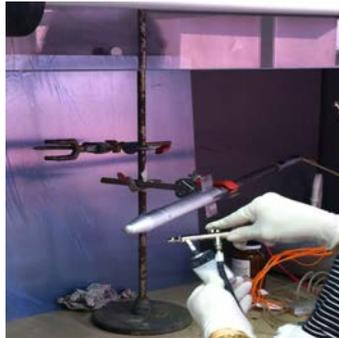
Figure 8. The VS-40 model being painted.
