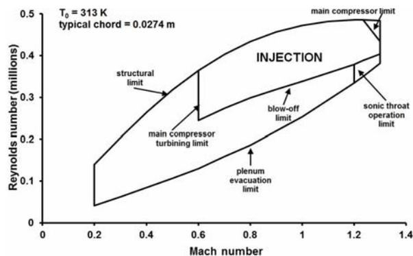
Figure 6. Operating envelope (injection system).
