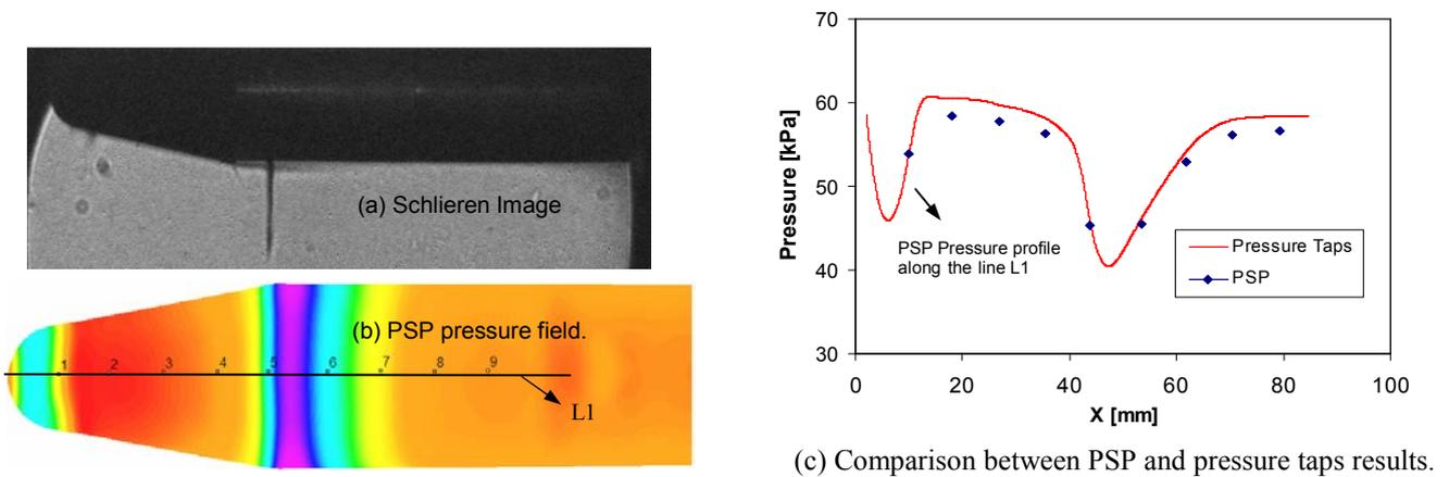
Figure 12. Schlieren and PSP results for Mach number equal to 0.9.
