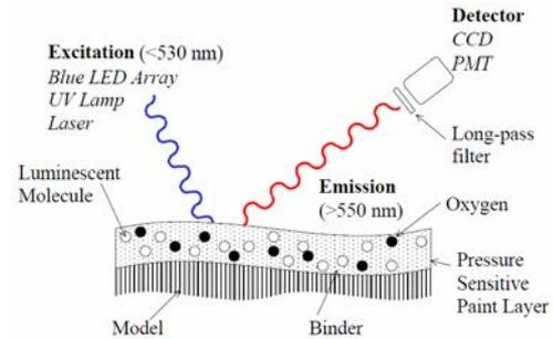
Figure 2. Basic Pressure-Sensitive.
