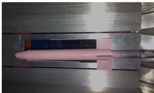
Figure 7. The VS-40 model painted with PSP paint inside the TTP test section.
