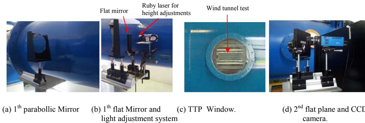
Figura 10. Schlieren /shadowgraph set-up.
