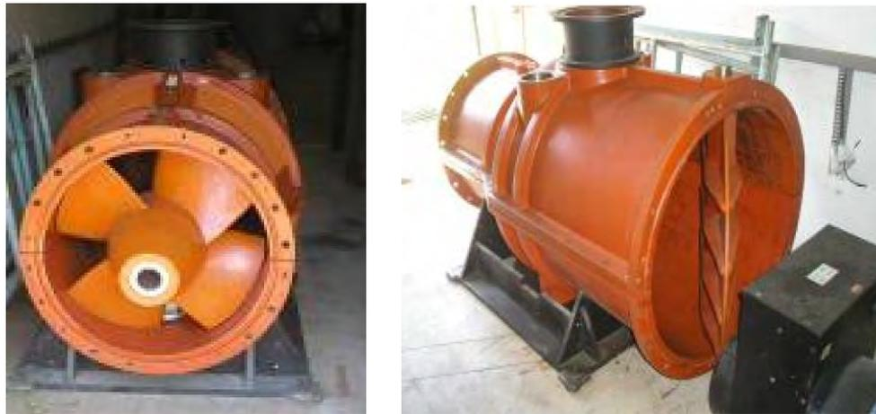
Figure 1. Views of the driving region of the axial-flow hydraulic turbine.
