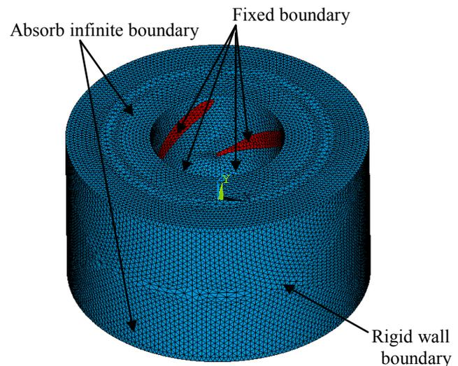
Figure 7. Turbine vanes meshed surrounded by water.
