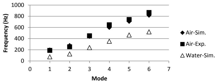
Figure 9. Natural frequencies in air (numerical e experimental) and water.
