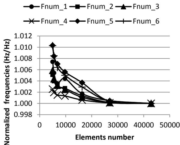
Figure 6. Results of the mesh sensitivity analysis.
