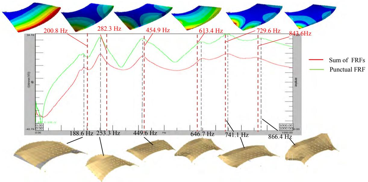
Figure 8. Vibrations modes of the runner vane in air by experimental analysis (bottom) and numerical analysis without adjustment (top).
