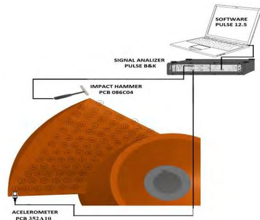
Figure 2. Flowchart adjustment Algorithm. Figure 3. Schematic of the test rig with the runner in air.
