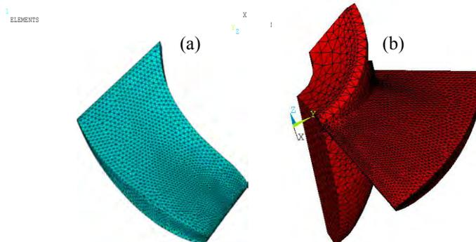
Figure 4. Turbine runner suspended by nylon. Figure 5. Turbine vane (a) and runner (b) meshed used on simulation.
