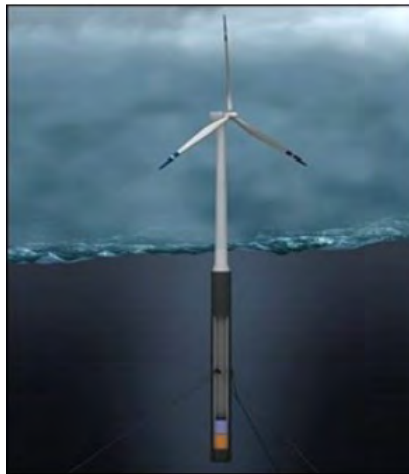
Figure 1. Floating Wind Turbine of Spar Type Hywind.
