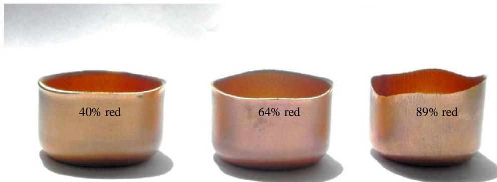
Figure 1. Deep drawn cups of the C22000 alloy. The thickness reduction by cold rolling of the original blank used for the cupping test is indicated in the photographs.
