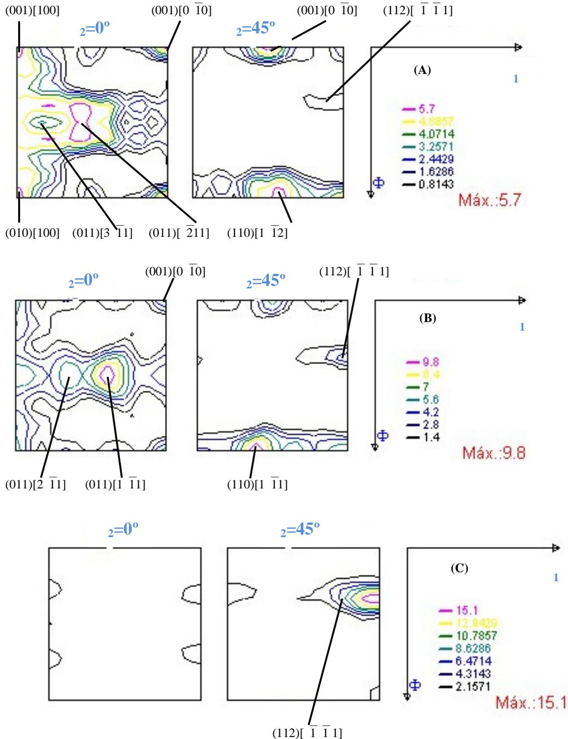
Figure 5. ODFs of the cold rolled samples with different thickness reductions: a) 45%; b) 64% and c) 89%..
