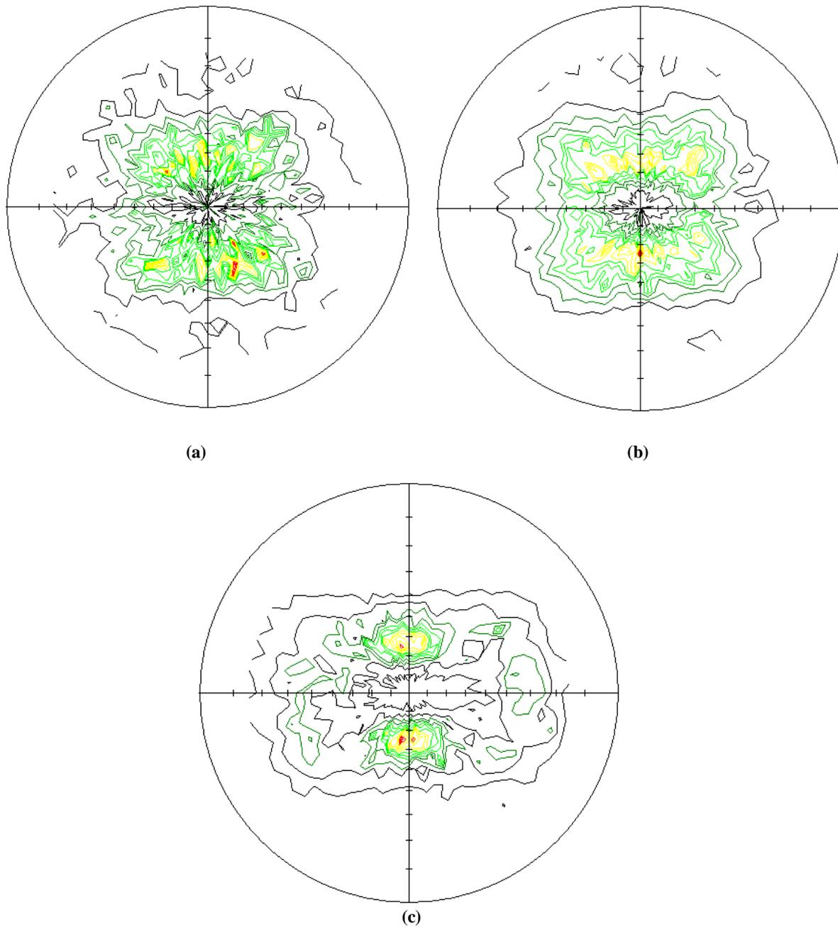
Figure 4. (111) pole figures of the ASTM C22000 alloy with different thickness reductions: a) 45%; b) 64% and c) 89%.
