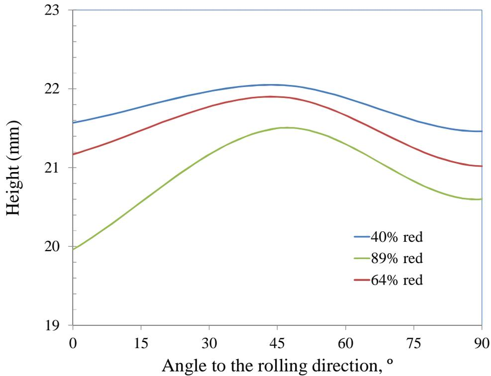
Figure 2. Earing profiles of the drawn cups with respect to the rolling direction.
