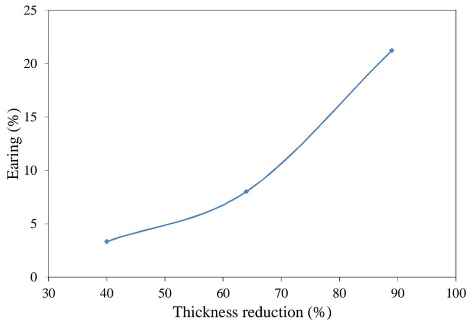
Figure 3. Earing percentage of the cups shown in Figure 1 plotted as a function of the thickness reduction.
