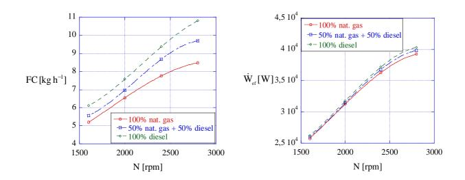
Figure 4. Fuel consumption and power simulation, Lintec 4LD 2500 engine, using natural gas and diesel
