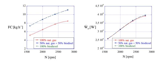
Figure 5. Fuel consumption and power simulation, Lintec 4LD 2500 engine, using natural gas and biodiesel
