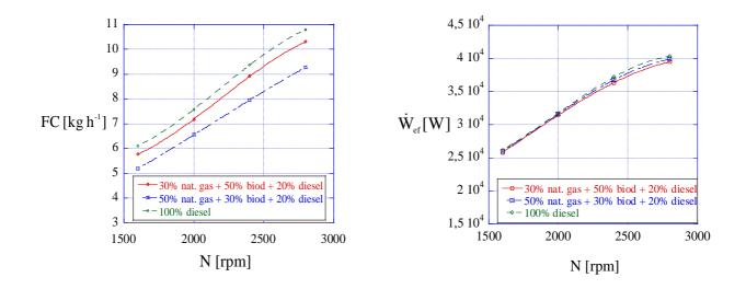
Figure 6. Fuel consumption and power simulation, Lintec 4LD 2500 engine, using natural gas, biodiesel and diesel
