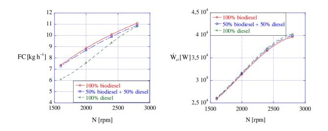
Figure 3. Fuel consumption and power simulation, Lintec 4LD 2500 engine, using biodiesel and diesel
