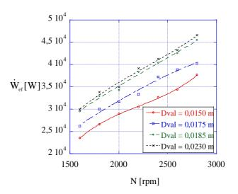
Figure 2. Power simulation, Lintec 4LD 2500 engine, with valve diameter variation
