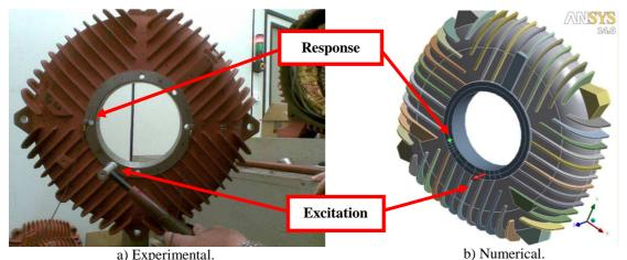
Figure 13 – Location example of the excitation and response points to obtain the FRF curves in the front end cover.
