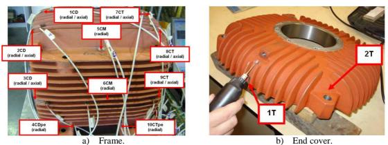
Figure 2 – Location and identification of the SG installed.
