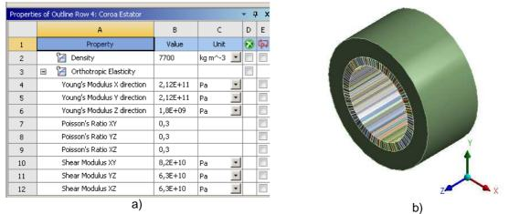
Figure 10 – Stator orthotropic data initially used into DX.
