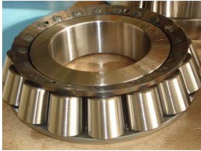
Figure 2. Conical bearing after repowering.
