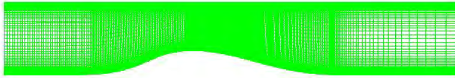
Figure 2. Overall view of the RANS mesh.
