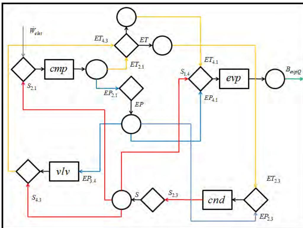
Figure 02: Productive structure of the refrigeration system of Fig. (1).
