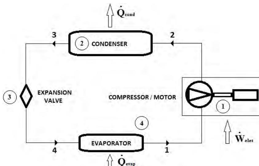
Figure 01: Simplified layout of the refrigeration system.
