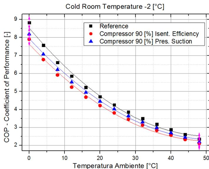
Figure 04: Impact in the COP due to malfunctions in the compressor.
