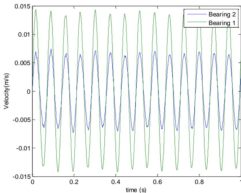
Figure 3 Simulated speeds the bearings 1 and 2.
