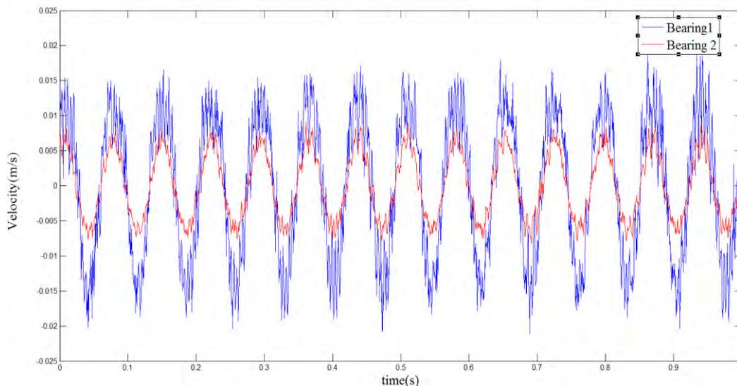
Figure 5. Experimental comparison velocity in the bearings.
