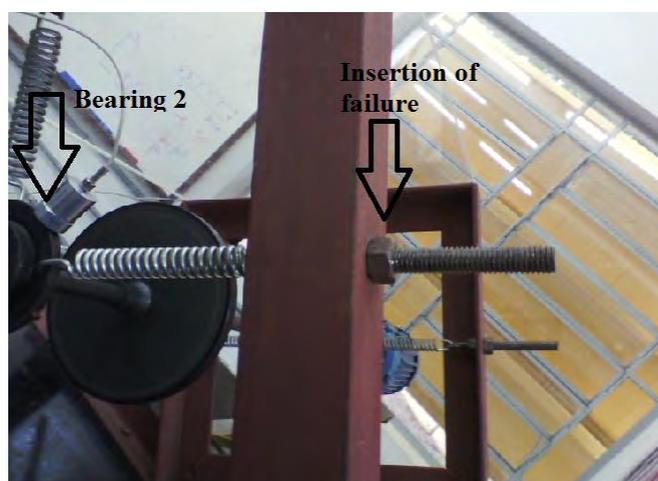
Figure 6. Mechanism for Fault Insertion.
