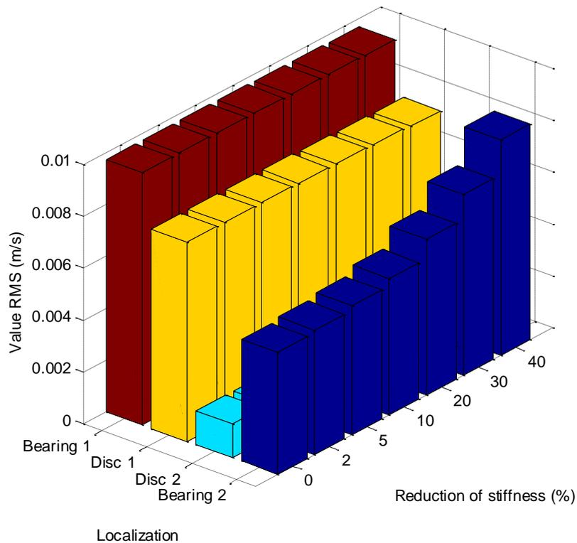
Figure 4. Influence of failures in RMS values.
