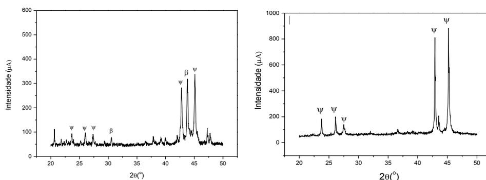
Figure 1. a) XRD of alloy after fusion quasicrystalina; b) diffraction after heat treatment for 12 hours.
