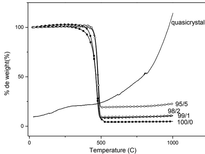
Figure 3. TGA thermograms of UHMWPE and its composites.
