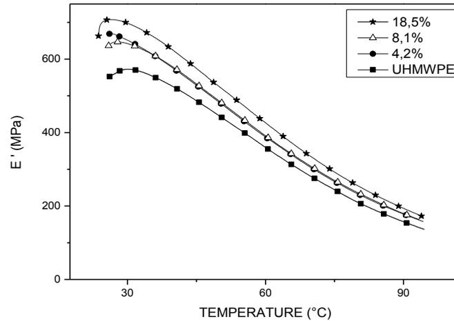
Figure 4- Storage Modulus curves of UHMWPE and its composites.
