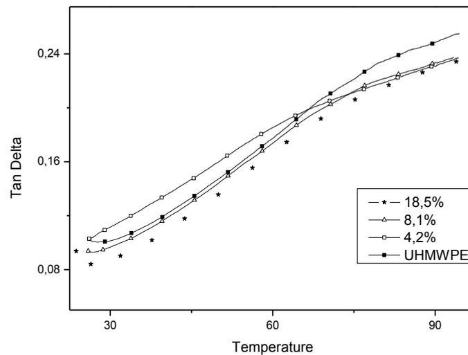
Figure 5. Tan  $\delta$  curves of UHMWPE and its composites.
