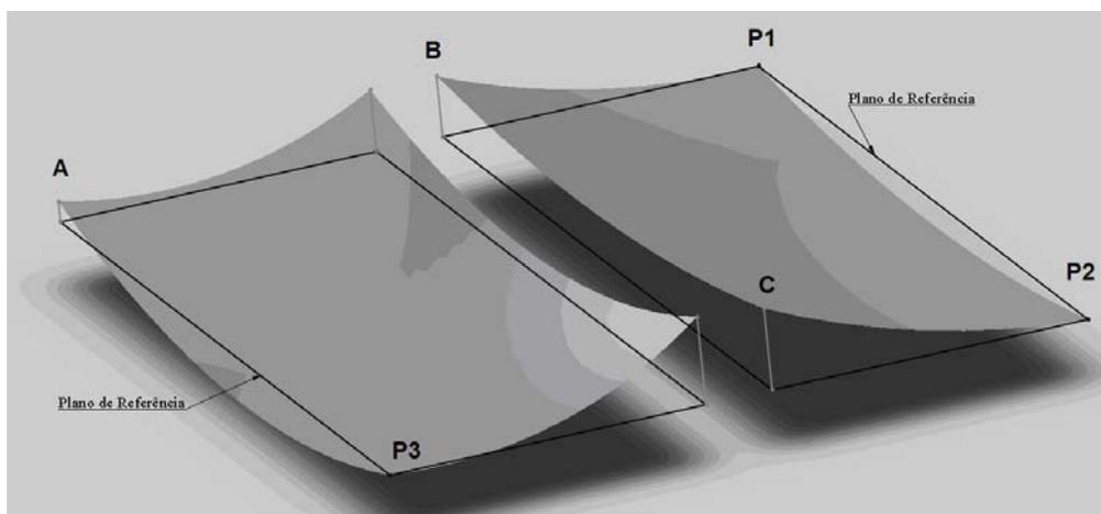
Figure 2. The reference plan and the control point positions A, B and C
