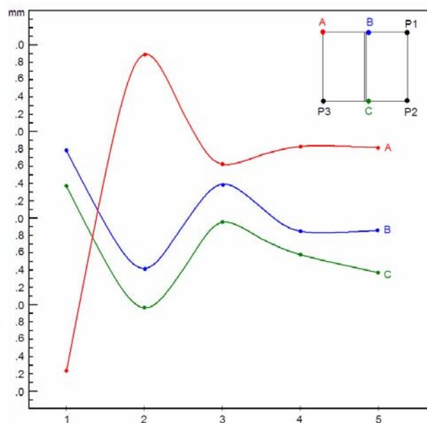
Figure 3. Vertical displacements of points A, B and C of the front surface of the welded plates for five days monitoring
