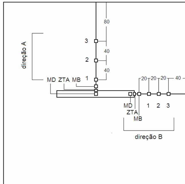
Figure 1. The location of the measurement points of the welding residual stress related to the repair welding
