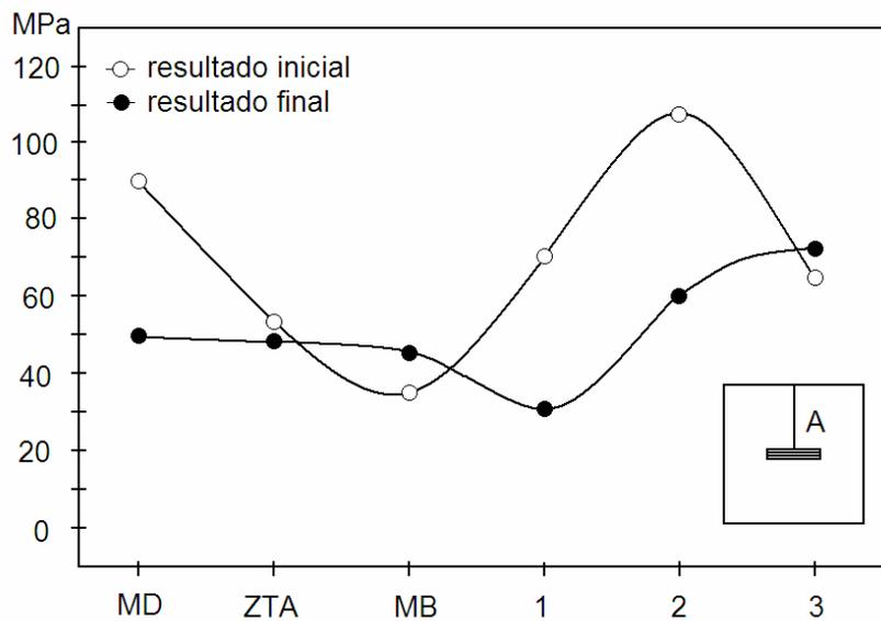
Figure 5. Direction A. Initial and finals values of maximum shear stress
