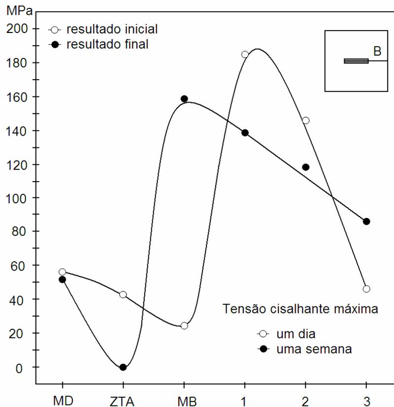
Figure 6. Direction B. Initial and final values of maximum shear stress
