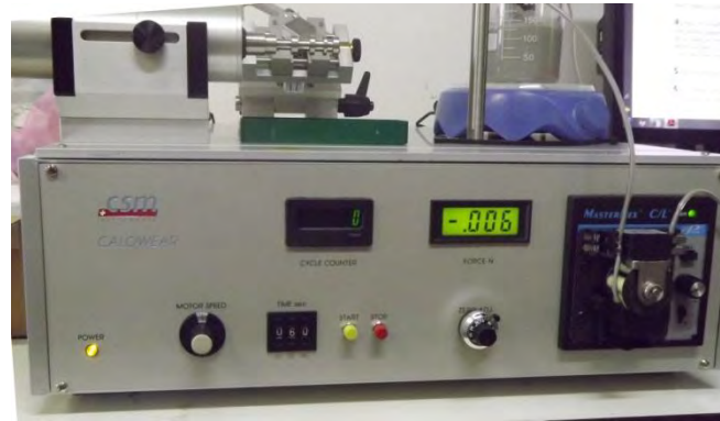
Figura 3 - Abrasive wear test equipment (CSM Calowear)
