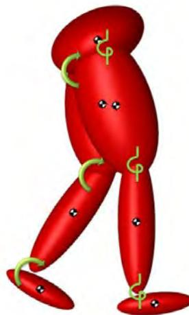
Figure 3. Single Support Underactuated Mechanism.
