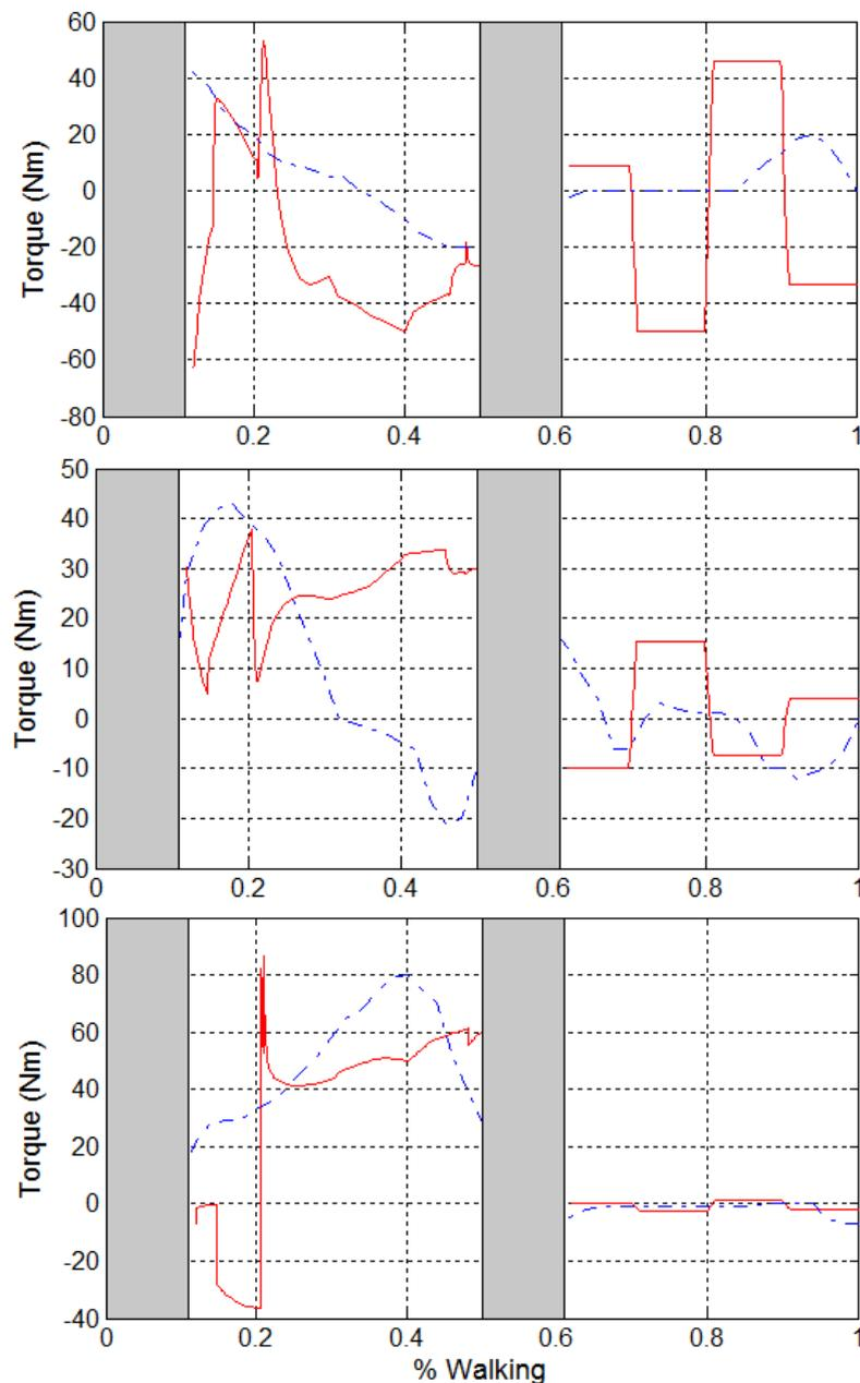
Figure 6 - Torques on hip, knee, and ankle joints, respectively, given by Chapman (dashed-dot lines) and given by the simulation (solid line).
