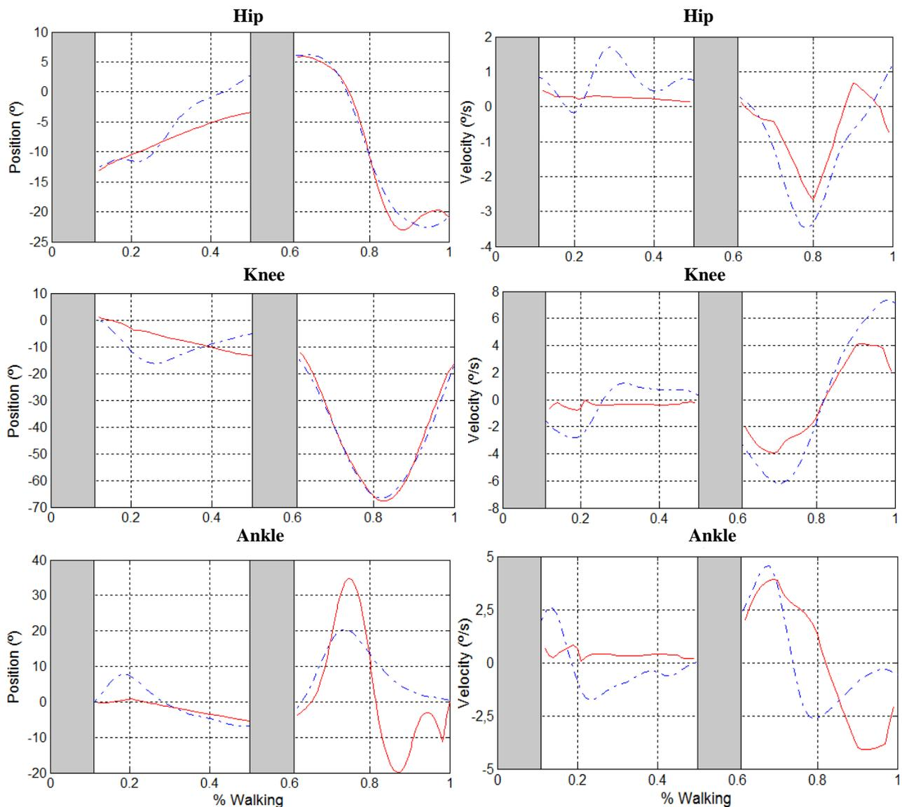
Figure 5. Position and Velocity on hip, knee, and ankle joints, respectively, given by Winter (dashed-dot lines) and given by the simulation (solid line).
