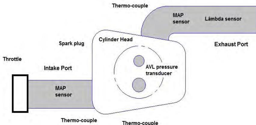
Figure 3. Engine installed sensors
