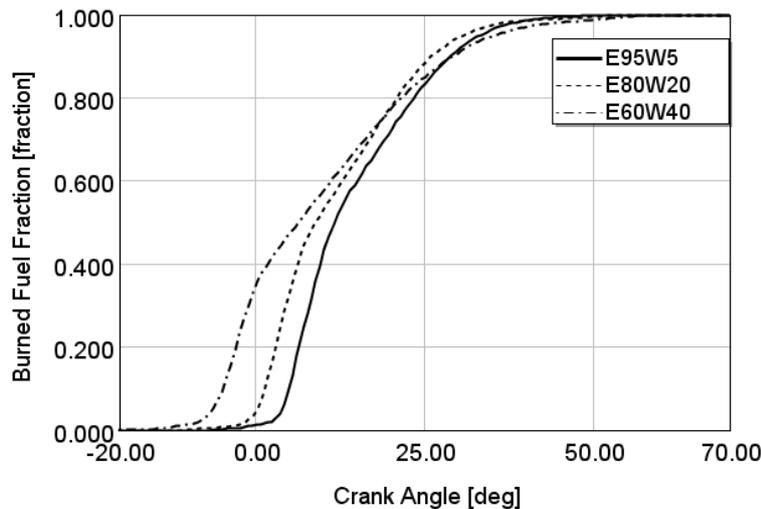
Figure 9. Burned fuel fraction of various fuel mixtures
