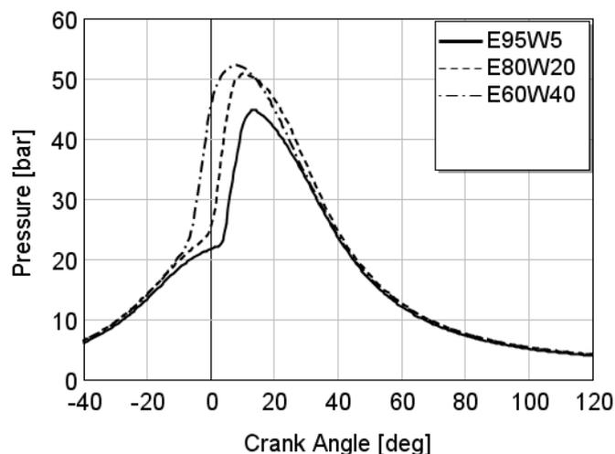
Figure 8. In-cylinder instantaneous pressure for different water-in-ethanol mixtures
