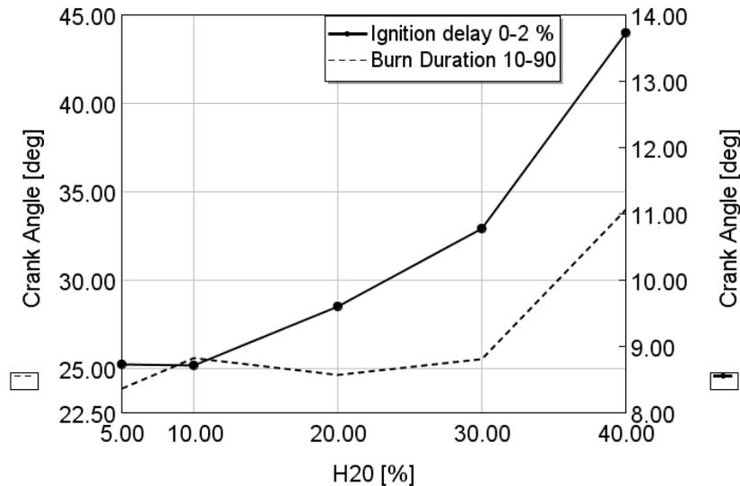
Figure 11. Burn duration 10-90% and ignition delay for different water-in-ethanol mixtures
