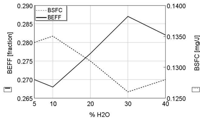
Figure 6. Engine Brake Efficiency and Brake Specific Fuel Consumption
