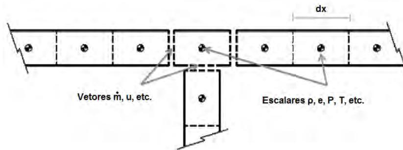
Figure 3. Discretization example of ducts used in GT-Power
