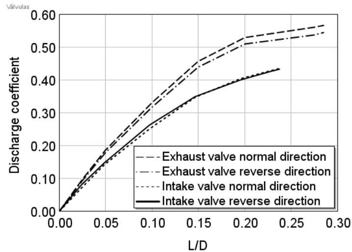
Figure 2. Discharge coefficient
