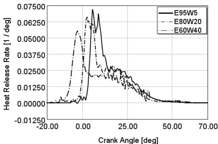
Figure 10. Heat release rates of fuel mixtures.
