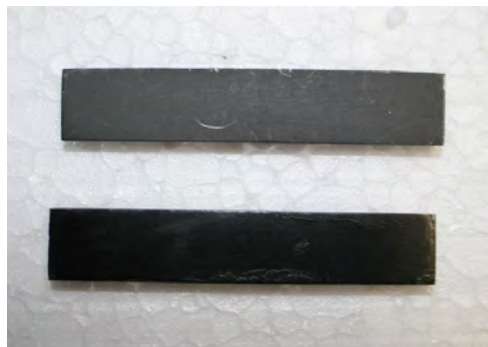
Figure 1. Samples painted with graphite powder (a) and with the ink conventional spray with bright finish (b).
