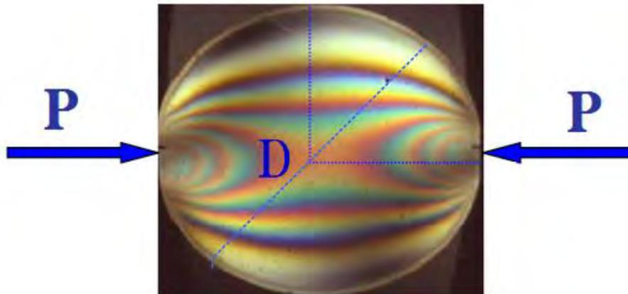
**Figure 8. Circular disk under compression loads**
