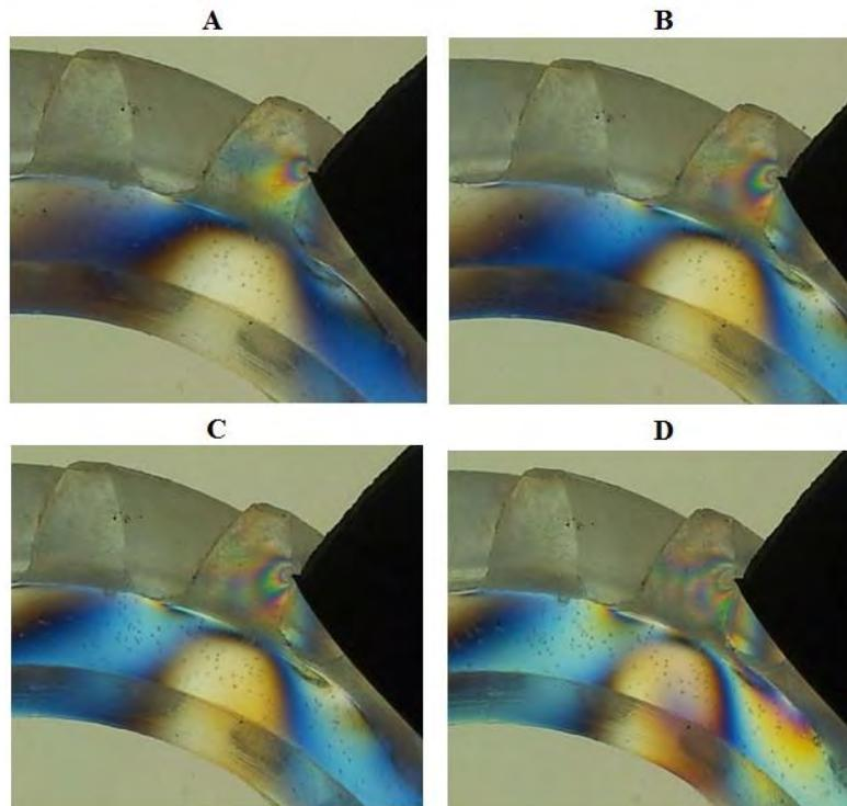
Figure 9. Fringe pattern for different values of moments applied
