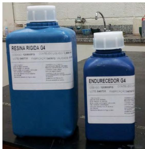
**Figure 5 - Epoxy resin of Polipox**
