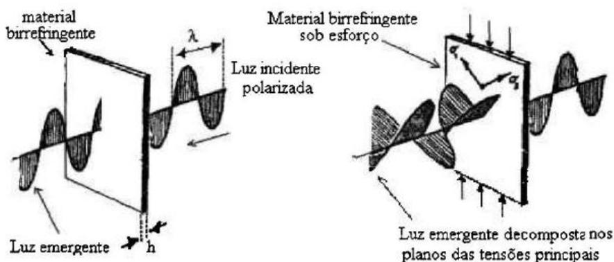
Figure 2. The phenomenon of birefringence mechanical
