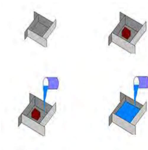
**Figure 4 - Method of manufacturing silicon molds**
