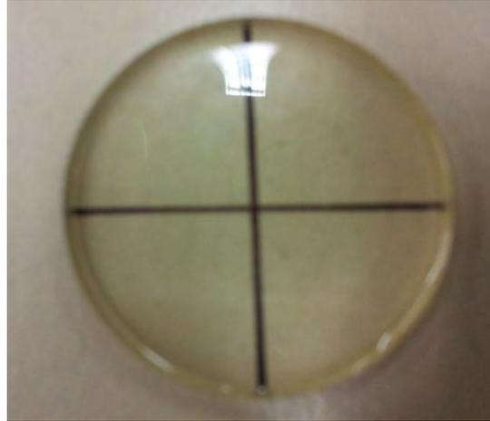
**Figure 7. Circular disc for calibration polariscope**
