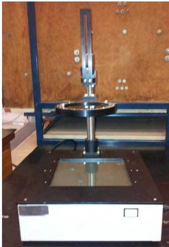
Figure 6. Polariscope
