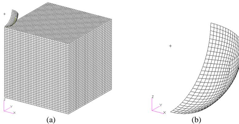
Figure 9. Finite element models: (a) workpiece modeled in one quarter; (b) spherical shell 0.1 mm thick, modeled in one half-quarter with rigid shell elements.
