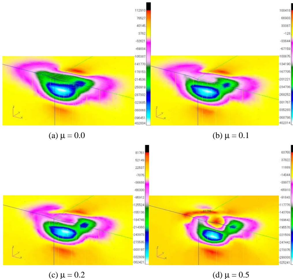
Figure 15. Influence of the friction coefficient for one oblique impact ( $\beta=30^\circ$ ) on the XX residual stress ( $v = 36 \text{ m/s}$ ;  $R = 0.7 \text{ mm}$ ;  $\mu = 0.2$ ;  $\alpha = 0.0012$ )
