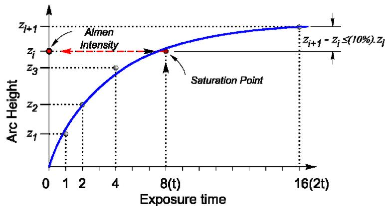
Figure 8. Saturation curve based on Almen tests.
