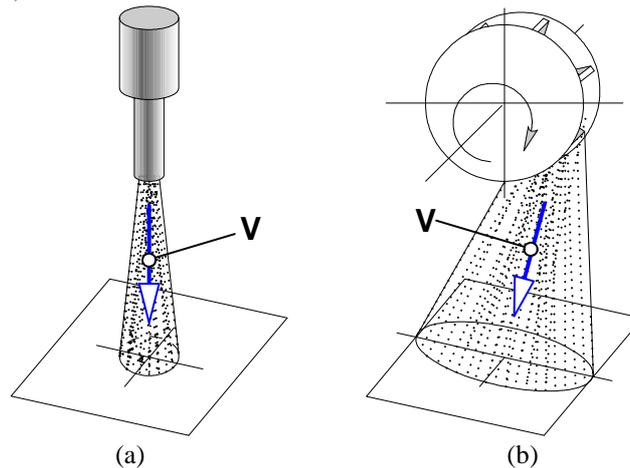
Figure 3. Some variations of SP principle: (a) air pressure; (b) centrifugal wheel.
