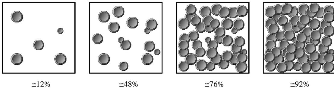
Figure 5. Number of indentations as a function of peening time.
