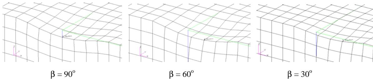
Figure 11. Effect of many oblique impacts of one sphere on the geometry deformation ( $v = 36$  m/s;  $R = 0.7$  mm;  $\mu = 0.2$ ).
