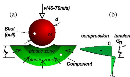
Figure 2. Shot peening: (a) impact of one shot; (b) distribution of residual stresses.
