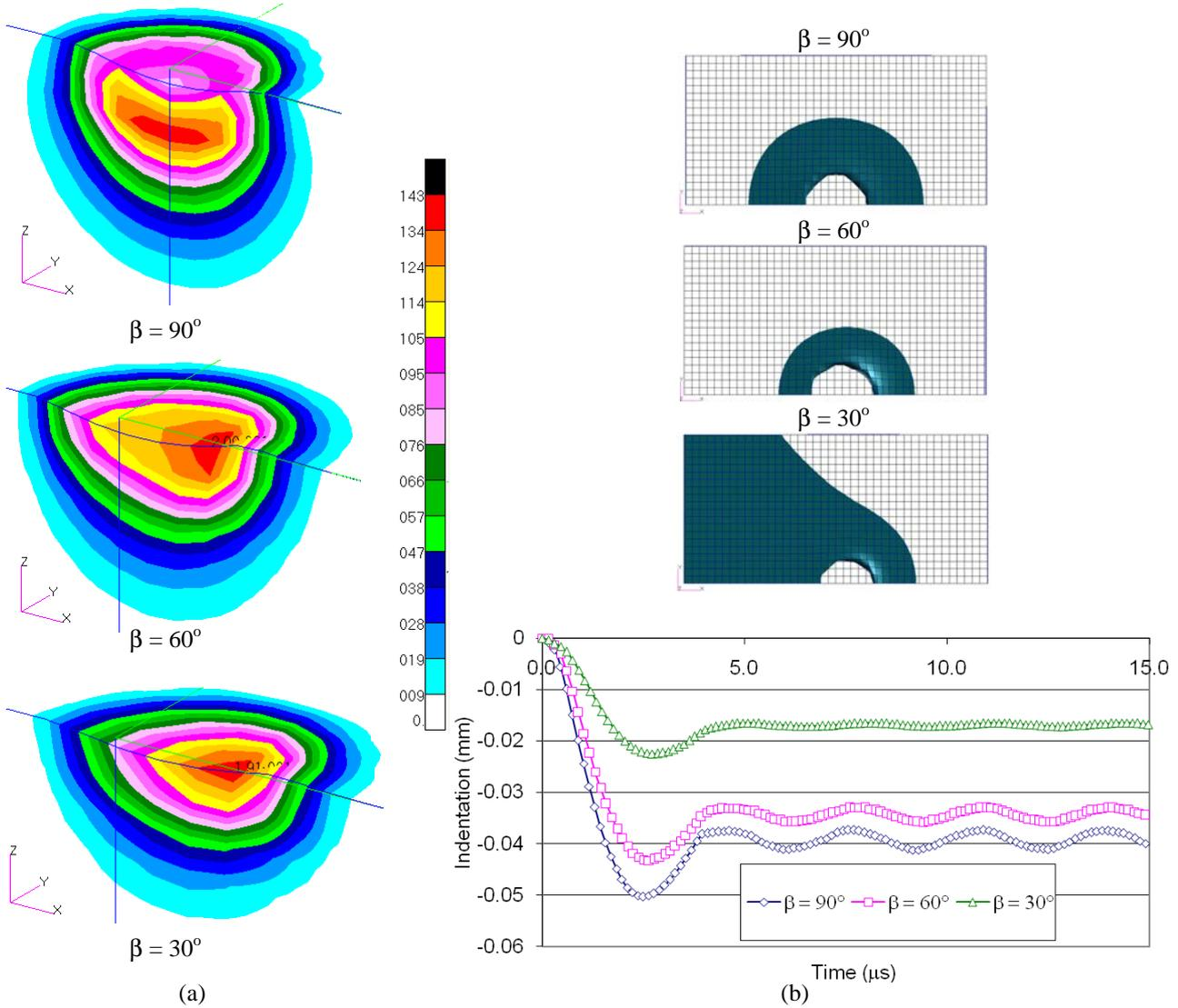
Figure 10. Effect of one single shot on: (a) equivalent plastic strain; (b) Z-displacement (indentation depth) ( $v = 36$  m/s;  $R = 0.7$  mm;  $\mu = 0.2$ ).
