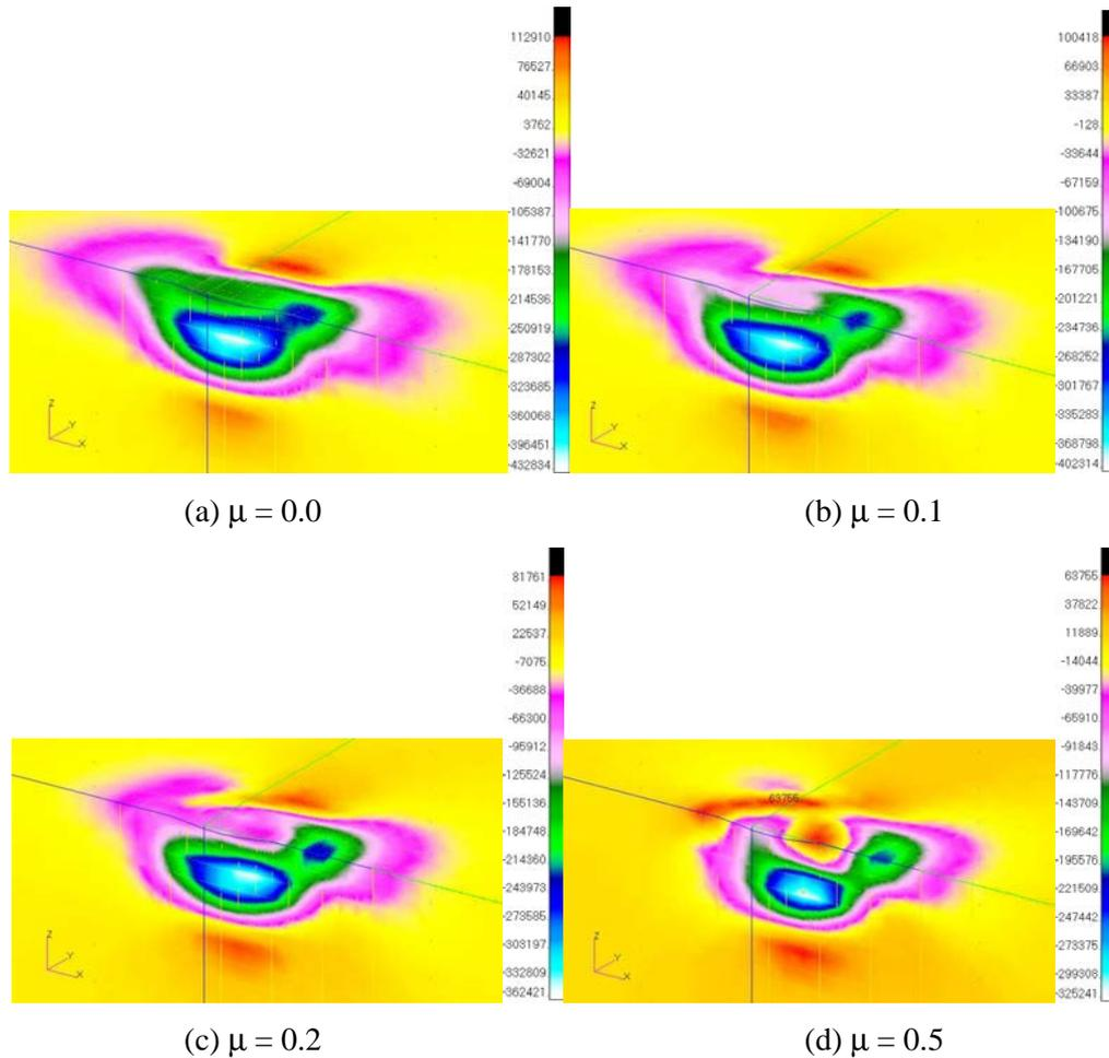
Figure 15. Influence of the friction coefficient for one oblique impact ( $\beta=30^\circ$ ) on the XX residual stress ( $v = 36$  m/s;  $R = 0.7$  mm;  $\mu = 0.2$ ;  $\alpha = 0.0012$ )
