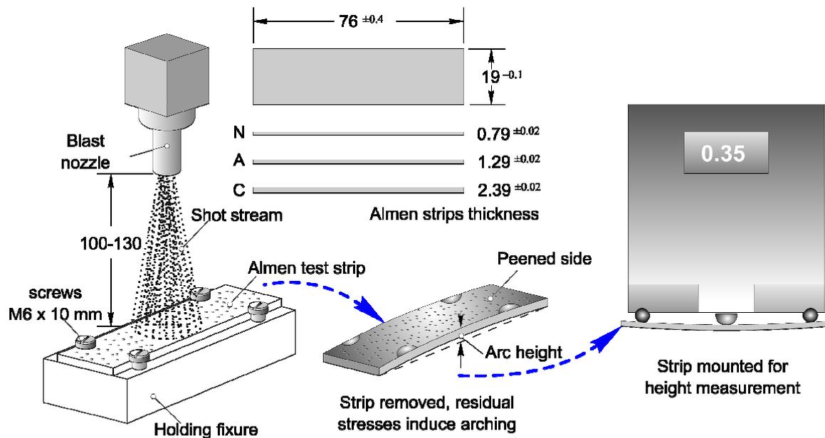
Figure 7. Almen strips deflected after shoot peening and measured with an Almen gauge.
