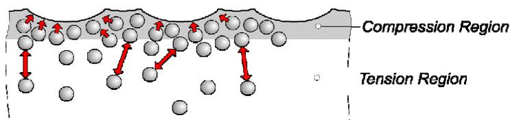
Figure 1. Shot peening at atomic level.
