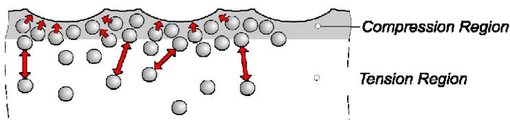
Figure 1. Shot peening at atomic level.
