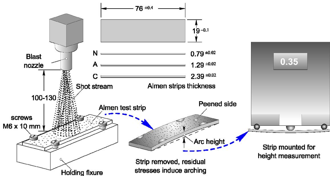
Figure 7. Almen strips deflected after shoot peening and measured with na Almen gauge.
