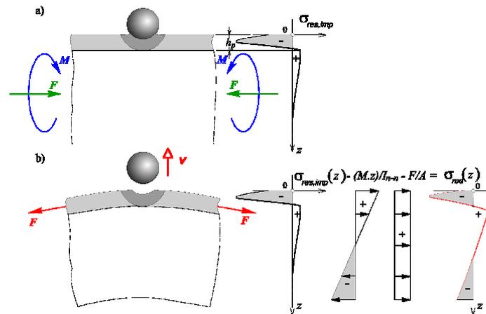
Figure 4. Determination of residual stress  $\sigma_{res}(z)$  for an Almen strip before (a) and after the removal of fixtures (b):
