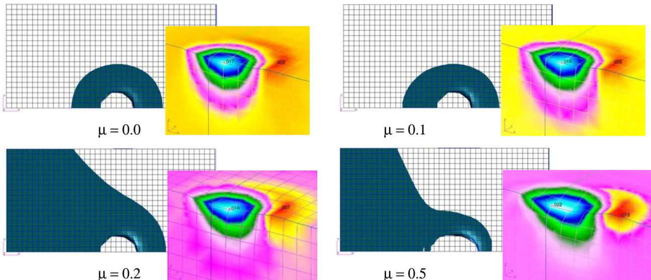
Figure 14. Influence of the friction coefficient for one oblique impact ( $\beta=30^\circ$ ) on the geometry deformation at the impact surface ( $v = 36$  m/s;  $R = 0.7$  mm;  $\mu = 0.2$ ;  $\alpha = 0.0012$ )
