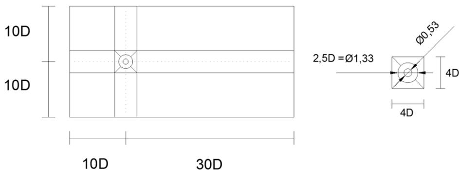
Figure 1. Computational domain for the numerical investigation
