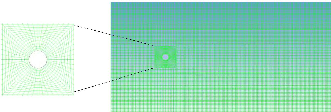
Figure 3. Numerical mesh applied to the cylinder
