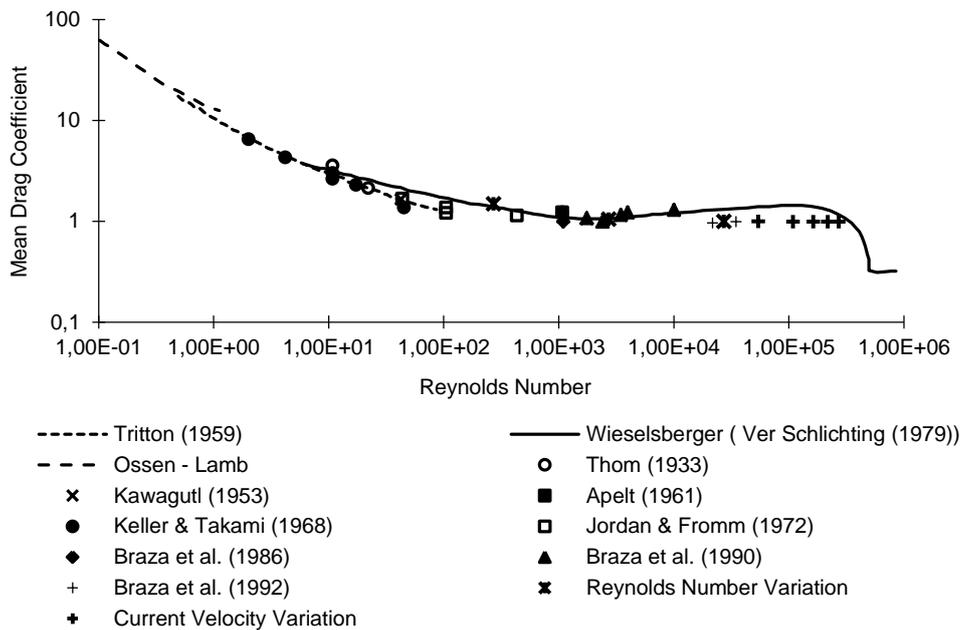
Figure 7. Mean drag coefficient for circular cylinder in steady current. Adapted from Sumer and Fredsoe (2006).
