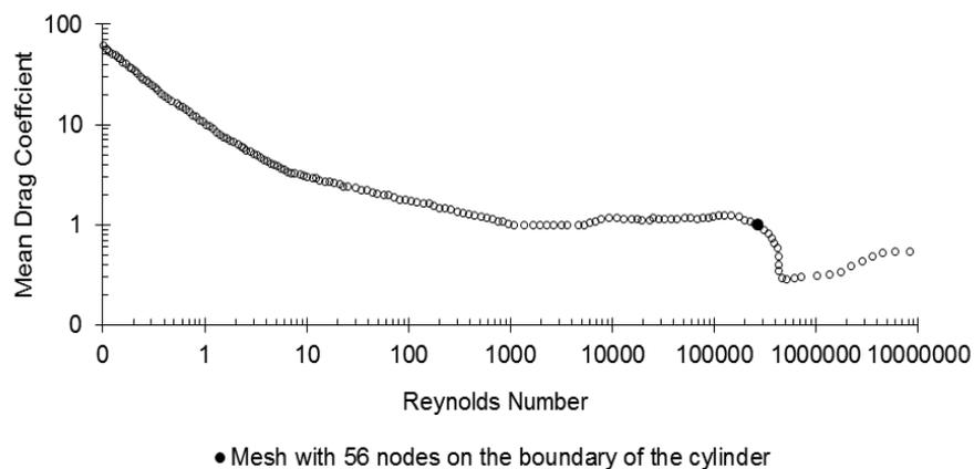
Figure 2. Resulting mean drag coefficient of the grid study convergence. Adapted from Sumer and Fredsoe (2006).
