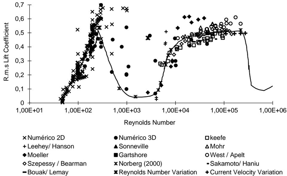
Figure 8. R.m.s lift coefficient versus Reynolds number. Adapted from Norberg (2003).
