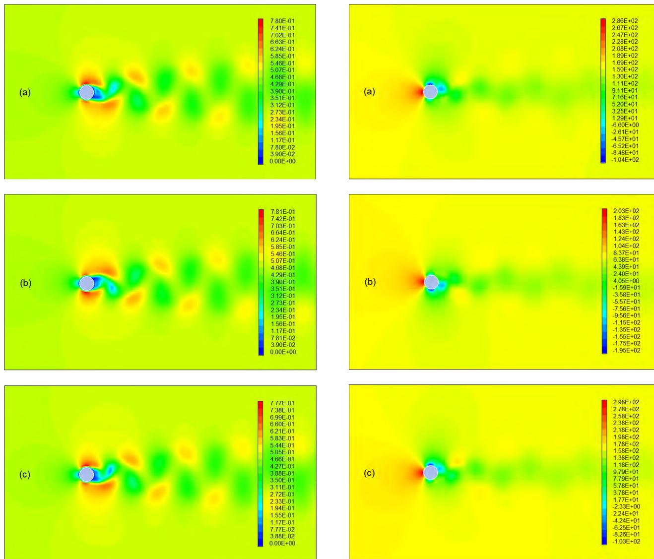
Figure 6. Contours of velocity magnitude (m/s) and static pressure (Pa). (a) Time=6.3900E+02. (b) Time=6.4113E+02. (c) Time=6.4326E+02
