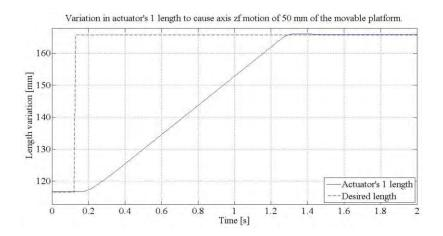
Figure 3. Variation in the length of the actuator 1 to cause motion in axis zf.
