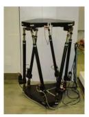
Figure 1. The Stewart platform of the Aerospace Control Laboratory.
