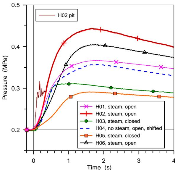
Figure 9. Containment pressures in EPR tests.
