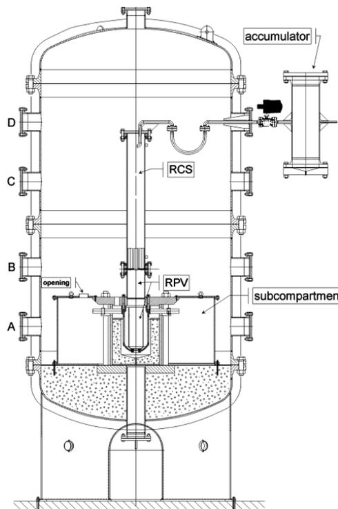
Figure 7. Scheme of the DISCO facility with the model of the EPR cavity.
