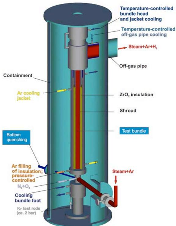
Figure 1. QUENCH containment and test section.
