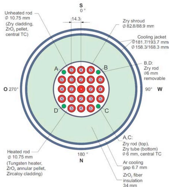
Figure 2. QUENCH bundle cross section.
