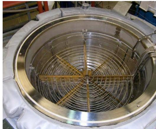
Figure 4. View of the LIVE-3D vessel with heating coils.
