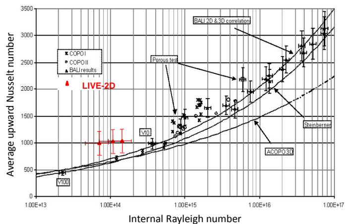
Figure 6. Comparison of the upward heat transfer in LIVE-2D tests with earlier experiments.
