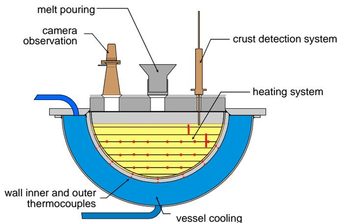
Figure 3. Scheme of the LIVE-3D test vessel.
