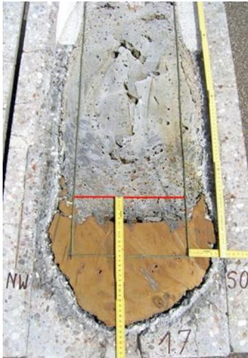
Figure 9. Cross-section of the MOCKA 1.7 crucible.
