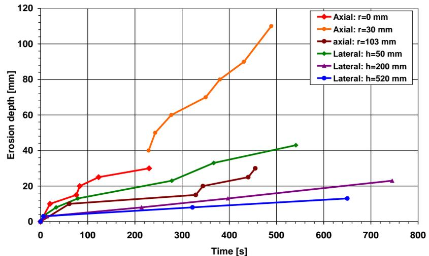
Figure 10. Position of the melt front as a function of time in the MOCKA 1.7 test.
