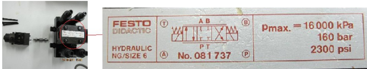
Figure 1: Hydraulic Proportional Valve.
