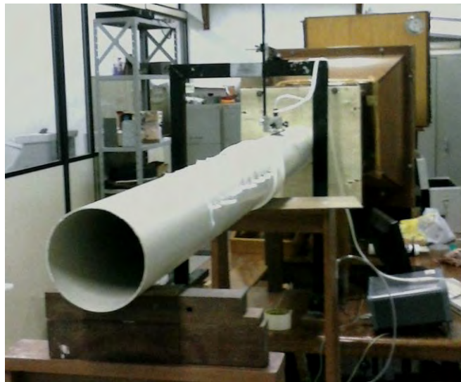
Figure 3. View of the PVC pipe coupled to a wind tunnel.
