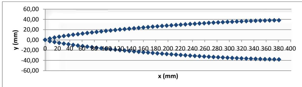
Figure 5. 100 points of the nose fairing profile using Von Karman shape equation Eq. 1
