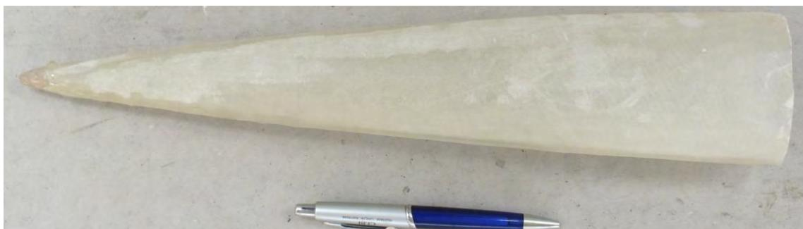
Figure 7. Fiberglass nose fairing based on Von Karman shape equation
