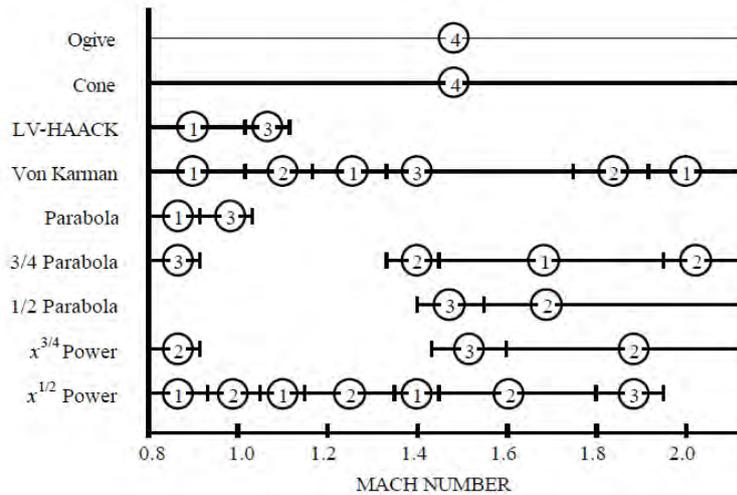
Figure 3. Comparison of drag characteristics of various nose shapes in the transonic-to-low Mach regions. Rankings are: Superior (1), Good (2), Fair (3), Inferior (4) (Crowell, 1996)
