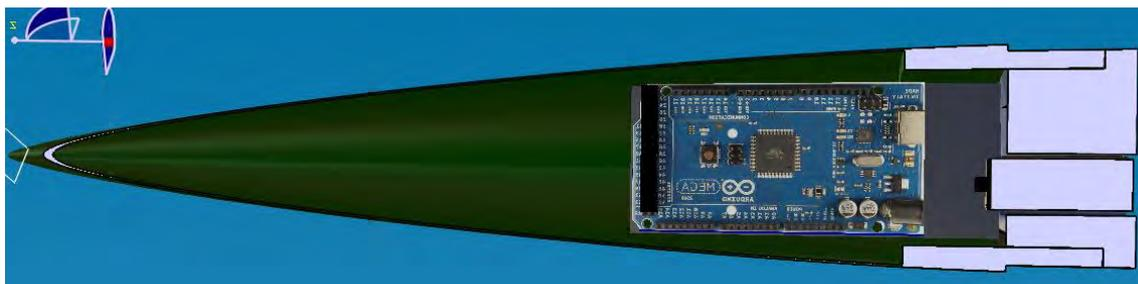
Figure 6. CAD drawing of the Von Karman nose fairing. The Cansat electronic is located inside the fairing because of the RF transparency characteristic of the fiberglass and to reduce the space needed of the payload part.
