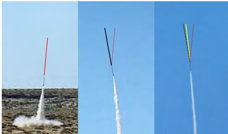
Figure 14. Deviation and recovery of the flight path during the 8<sup>th</sup> IREC
