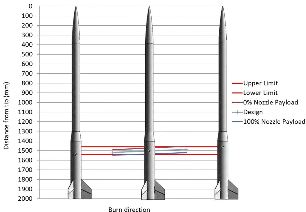
Figure 11. Designed Center of Gravity inside the finset limits for a statically stable rocket
