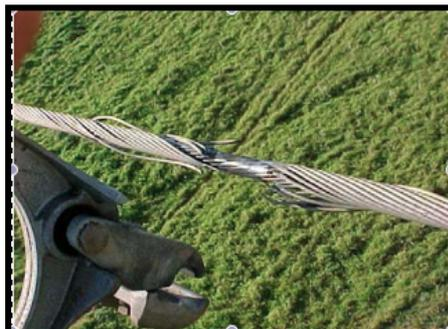
Figure 1 – Typical fatigue failure in overhead conductors, (Cigrè, 2006).
