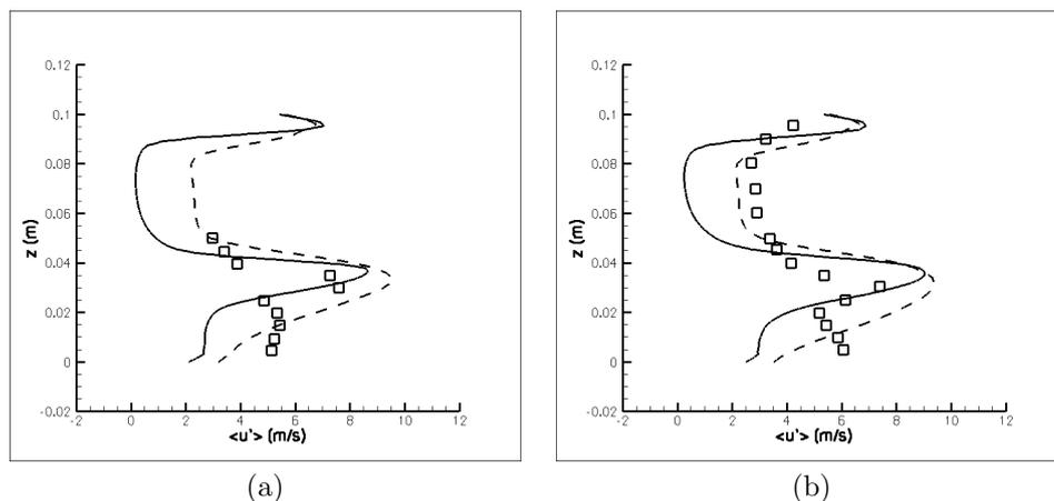
Figure 4. Mean velocity fluctuations obtained from the application of the turbulence model proposed by Germano *et al.* (1991) and the RFG method for the inlet turbulent conditions: (a)  $x_m = 0.08\text{ m}$  and (b)  $x_m = 0.10\text{ m}$ . □ Moreau *et al.* (1996), — Dynamic Smagorinsky's model and - - - Dynamic Smagorinsky's model with RFG.
