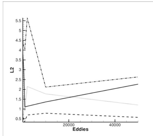
Figure 5. Influence of the quantity of generated eddies and the characteristic length determination proposition in the  $L_2$  norm. — case A, - - - case B, - · - case C and ··· case D
