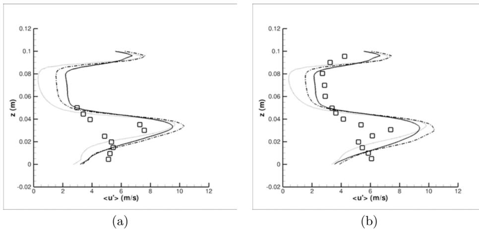
Figure 10. Mean velocity fluctuations obtained from the application of the turbulence model proposed by Germano *et al.* (1991) and the use of SEM and RFG methods for the inlet turbulent conditions: (a)  $x_m = 0.08 m$  and (b)  $x_m = 0.10 m$ .  $\square$  Moreau *et al.* (1996), — RFG,  $\cdots$  SEM - case B, - - - SEM - case D.
