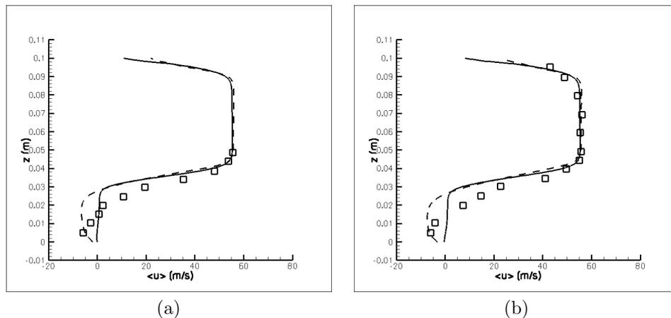
Figure 1. Mean velocity profiles obtained from the application of the turbulence models proposed by Smagorinsky (1963) and Germano *et al.* (1991): (a)  $x_m = 0.08\text{ m}$  and (b)  $x_m = 0.10\text{ m}$ .  $\square$  Moreau *et al.* (1996), — Classical Smagorinsky's model and - - - Dynamic Smagorinsky's model.
