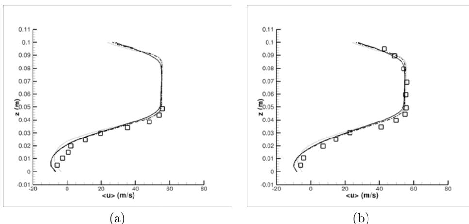
Figure 9. Mean velocity profiles obtained from the application of the turbulence model proposed by Germano *et al.* (1991) and the use of SEM and RFG methods for the turbulent inlet conditions: (a)  $x_m = 0.08 m$  and (b)  $x_m = 0.10 m$ .  $\square$  Moreau *et al.* (1996), — RFG, ··· SEM - case B, - - - SEM - case D.
