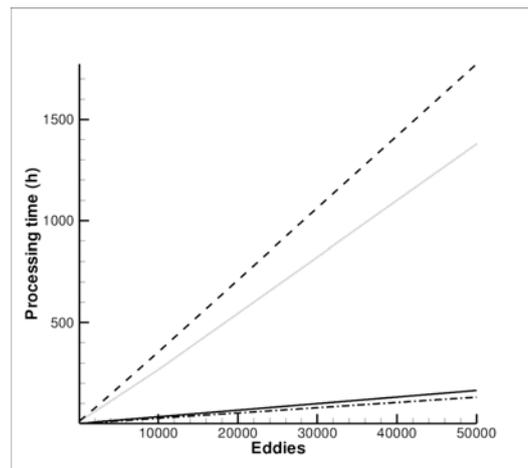
Figure 6. Influence of the quantity of generated eddies and the characteristic length determination proposition in the processing time required by the proposed methodology. — case A, - - - case B, - · - case C and · · · case D.
