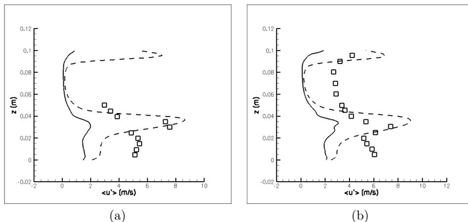
Figure 2. Mean velocity fluctuations, obtained from the application of the turbulence models proposed by Smagorinsky (1963) and Germano *et al.* (1991): (a)  $x_m = 0.08\text{ m}$  and (b)  $x_m = 0.10\text{ m}$ .  $\square$  Moreau *et al.* (1996), — Classical Smagorinsky's model and - - - Dynamic Smagorinsky's model.
