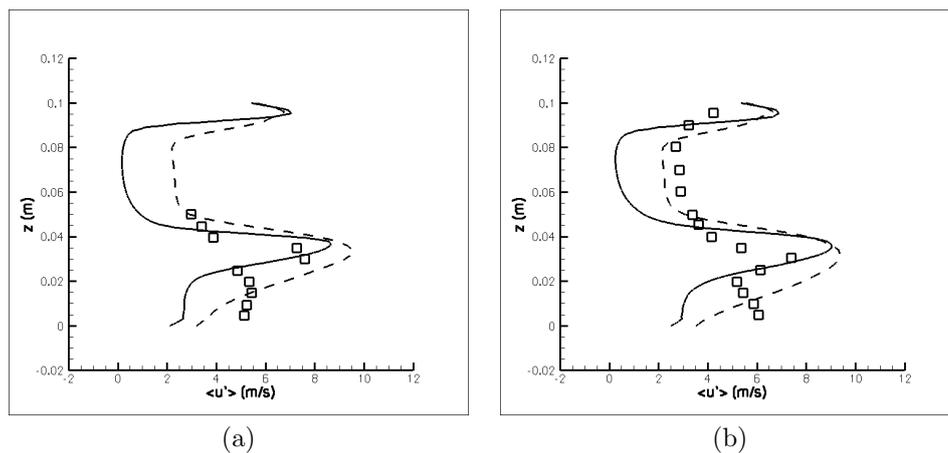
Figure 4. Mean velocity fluctuations obtained from the application of the turbulence model proposed by Germano *et al.* (1991) and the RFG method for the inlet turbulent conditions: (a)  $x_m = 0.08\text{ m}$  and (b)  $x_m = 0.10\text{ m}$ .  $\square$  Moreau *et al.* (1996), — Dynamic Smagorinsky's model and - - - Dynamic Smagorinsky's model with RFG.
