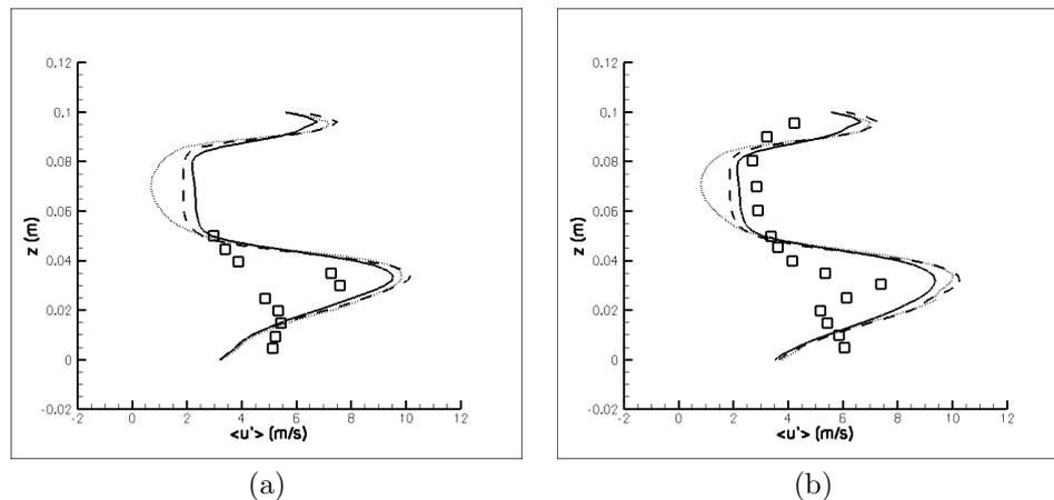
Figure 8. Mean velocity fluctuations obtained from the application of the turbulence model proposed by Germano *et al.* (1991) and the use of SEM and RFG methods for the inlet turbulent conditions: (a)  $x_m = 0.08 m$  and (b)  $x_m = 0.10 m$ .  $\square$  Moreau *et al.* (1996), — RFG, - - - SEM - 10000 eddies, - · - SEM - 100000 eddies.
