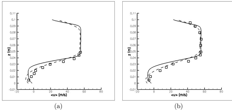
Figure 3. Mean velocity profiles obtained from the application of the turbulence model proposed by Germano *et al.* (1991) and the RFG method for the inlet turbulent conditions: (a)  $x_m = 0.08\text{ m}$  and (b)  $x_m = 0.10\text{ m}$ .  $\square$  Moreau *et al.* (1996), — Dynamic Smagorinsky's model and - - - Dynamic Smagorinsky's model with RFG.
