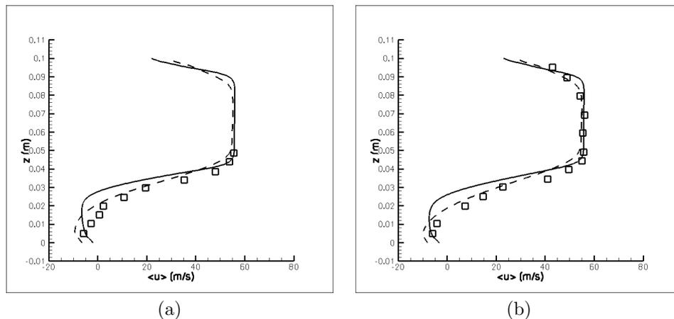
Figure 3. Mean velocity profiles obtained from the application of the turbulence model proposed by Germano *et al.* (1991) and the RFG method for the inlet turbulent conditions: (a)  $x_m = 0.08\text{ m}$  and (b)  $x_m = 0.10\text{ m}$ . □ Moreau *et al.* (1996), — Dynamic Smagorinsky's model and - - - Dynamic Smagorinsky's model with RFG.
