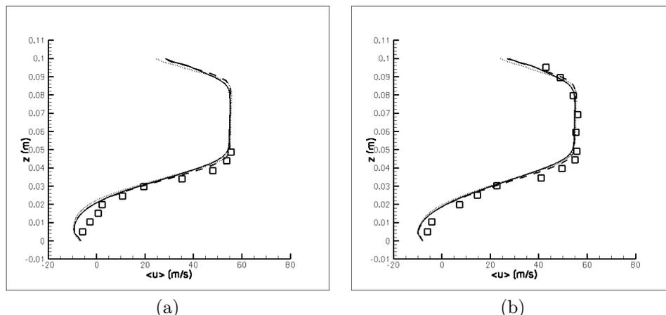
Figure 7. Mean velocity profiles obtained from the application of the turbulence model proposed by Germano *et al.* (1991) and the use of SEM and RFG methods for the turbulent inlet conditions: (a)  $x_m = 0.08$  m and (b)  $x_m = 0.10$  m.  $\square$  Moreau *et al.* (1996), — RFG, - - - SEM - 10000 eddies, - · - SEM - 100000 eddies.
