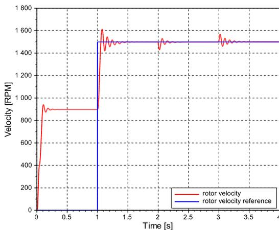
Figure 14. DMC load response:  $\omega_r$ .
