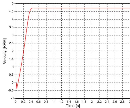
Figure 5. Step response from  $\omega_e$  to  $\omega_r$ .
