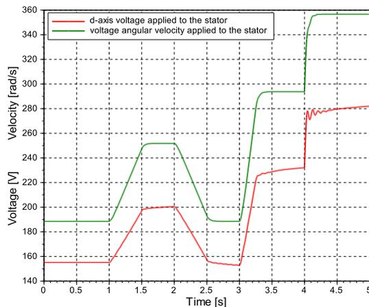
Figure 18. SSMPC response:  $v_{ds}$  and  $\omega_e$ .
