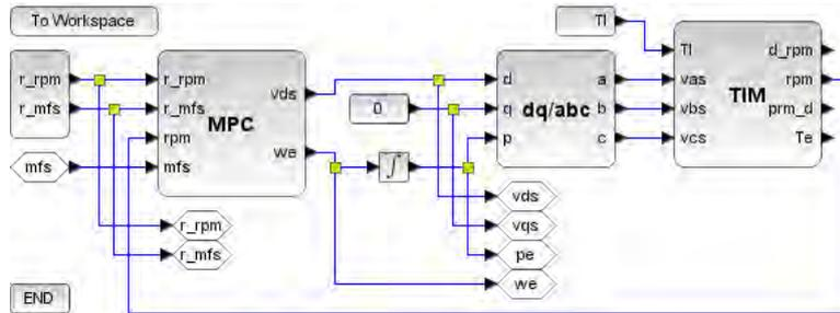
Figure 2. Environment used to emulate a TIM MPC loop.
