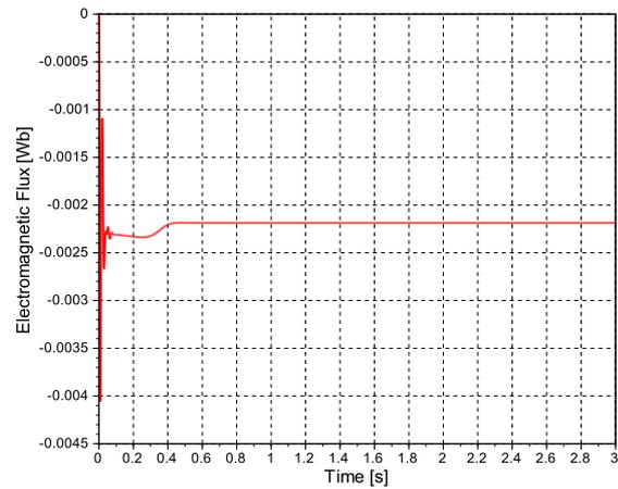
Figure 7. Step response from  $\omega_e$  to  $|\lambda_s|$ .
