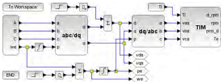
Figure 3. Environment used to obtain the TIM step response.
