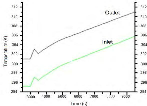
Figure 5. Inlet and Outlet core coolant temperature predicted by RELAP5/MOD3.3 after forced recirculation off at 3000 s.
