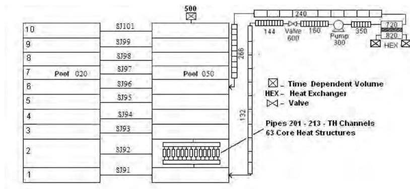
Figure 2. IPR-R1 Modeling using the RELAP5.
