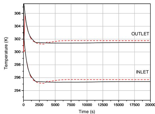
Figure 4. Coolant temperature evolution for channel 1 of the IPR-R1 at 100 kW of power operation for RELAP5-3D (dash red line) and RELAP5/MOD3.3 (straight black line) models.
