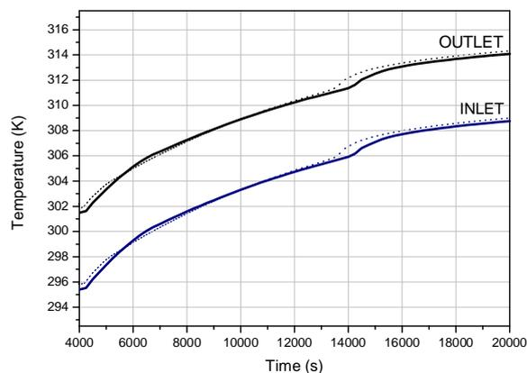
Figure 6. Core inlet and outlet temperatures increasing after the decrease of the pump velocity beginning at 4000 s of calculation at 100 kW for RELAP5-3D (dash line) and RELAP5/MOD3.3 (straight line) models.
