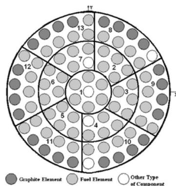
Figure 3. Core nodalization in RELAP5 showing the 13 TH channels.
