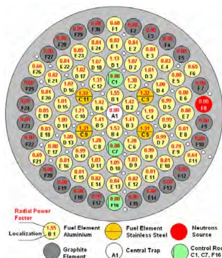
Figure 1. Core radial relative power distribution.
