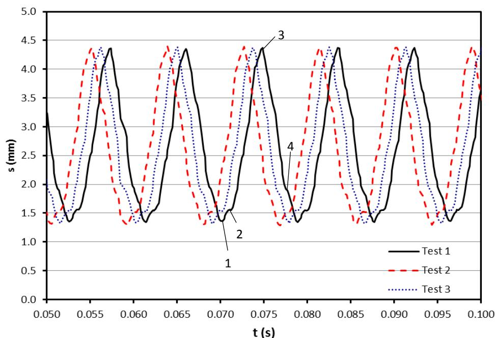
Figure 4 – Instantaneous displacement of the reed,  $s$
