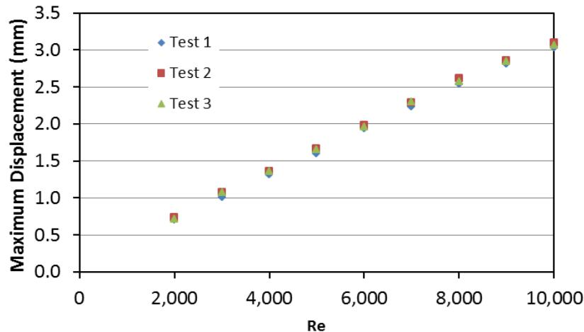
Figure 6 – Maximum displacement (s) of the reed as a function of the Reynolds number
