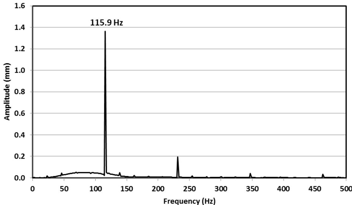
Figure 5 – Fast Fourier Transform of the instantaneous displacement signal
