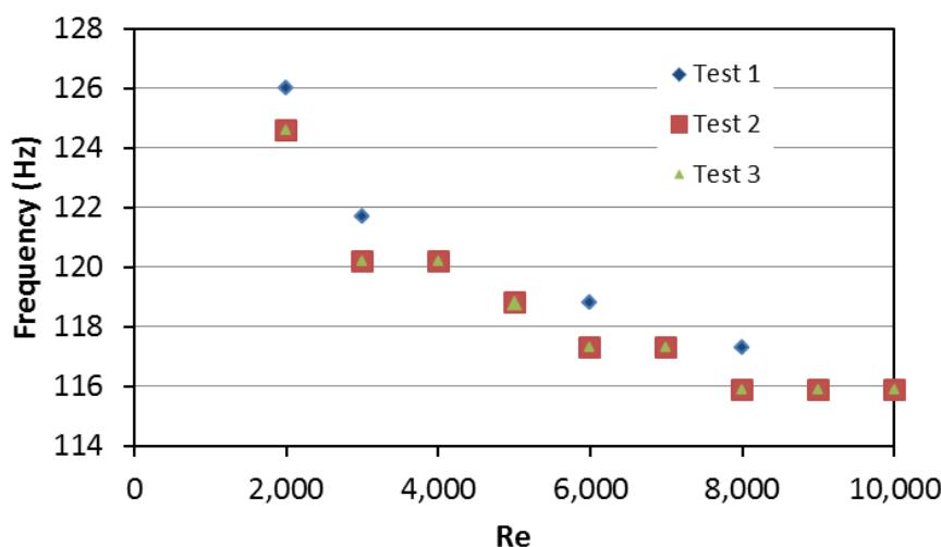
Figure 5 – Frequency of the reed movement as a function of the reynolds number
