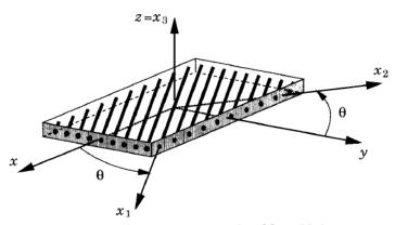
Figure 1. Laminate fiber orientation. (Reddy, 1997)
