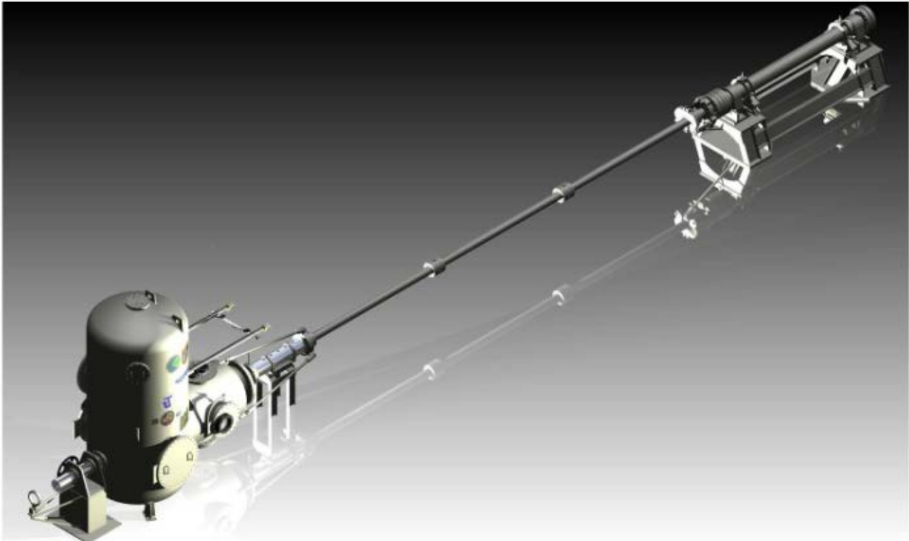
Figure 14: T3 0.60-m. nozzle exit diameter Hypersonic Shock Tunnel.
