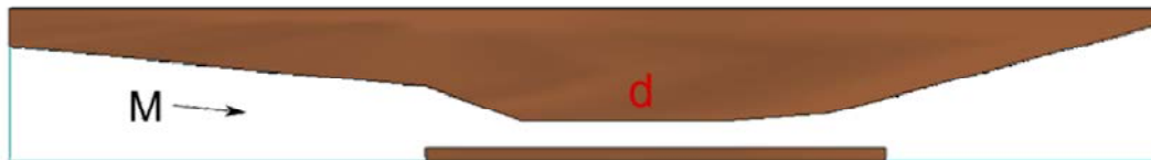
Figure 9: The truncated 14-X waverider scramjet Mach number 10 model concept.
