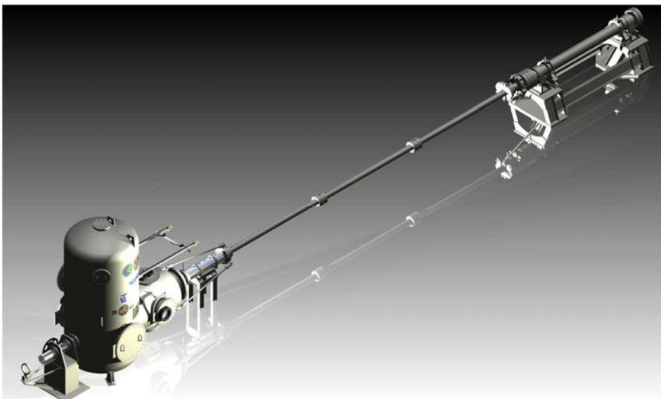
Figure 2: T3 0.60-m. nozzle exit diameter Hypersonic Shock Tunnel.
