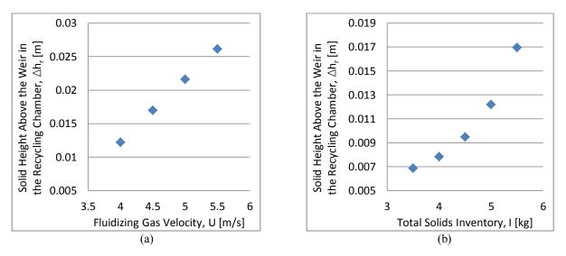
Figure 5 – Solid height above the weir in the recycle chamber,  $\Delta h_r$ :(a) with the varying the fluidizing velocity; (b) with the variation of the inventory of solids.
