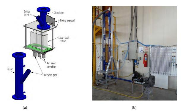
Figure 1– (a) Loop-seal (a); (b) CFFU used in experimental tests.
