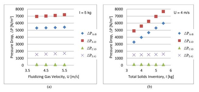
Figure 3 - Pressure drop in the fluidization loop. (a) Variation with the fluidizing gas velocity; (b) Variation with the total solids inventory.
