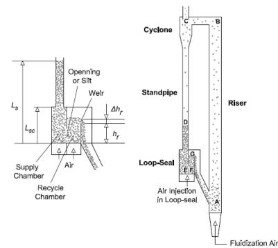
Figure 1 - CFB system with loop-seal details. Adapted from Basu and Cheng (2000).
