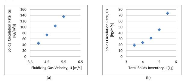
Figure 4 – Solids circulation rate behavior, Gs:(a) Variation of the fluidizing velocity; (b) Variation of the solids inventory.
