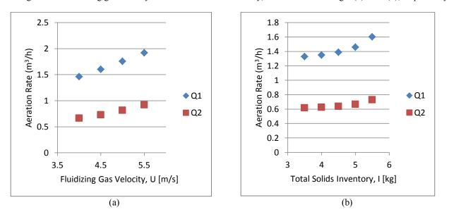
Figure 6 – Aeration rate in the supply chamber (Q<sub>1</sub>) and in the recycle chamber (Q<sub>2</sub>). (a) Variation of the fluidizing gas velocity; (b) Variation of the total solids inventory.
