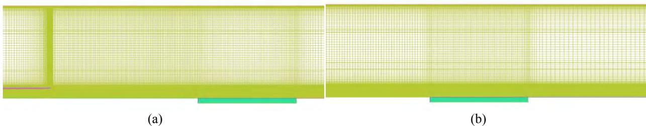
Figure 3. Sample grid refinement: (a) at jet orifice exit region and (b) around heated region.
