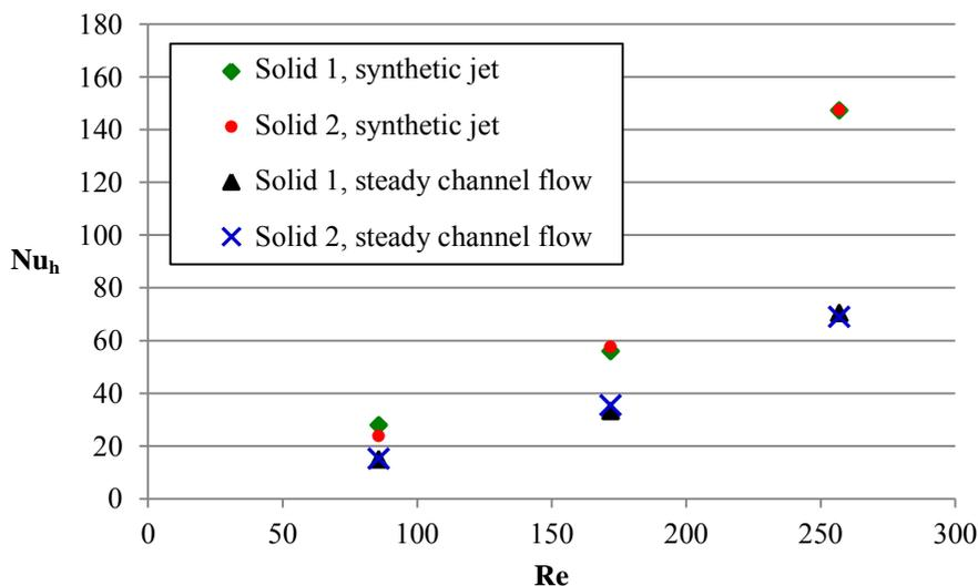
Figure 5.  $Nu_h$  vs.  $Re$  for both Solid configurations and  $2St$  case.
