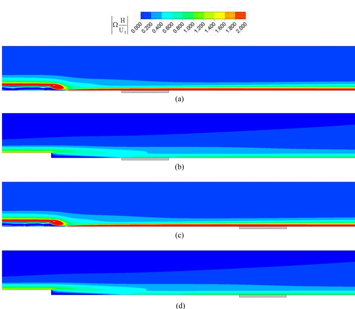
Figure 6. Time-averaged normalized absolute vorticity contours ( $Re = 172$ ,  $St_{U_0} = 0,041$ ) for (a) Solid 1 over the 10th pulsing cycle; (b) Solid 1 with steady channel flow; (c) Solid 2 over the 10th pulsing cycle; (d) Solid 2 with steady channel flow.
