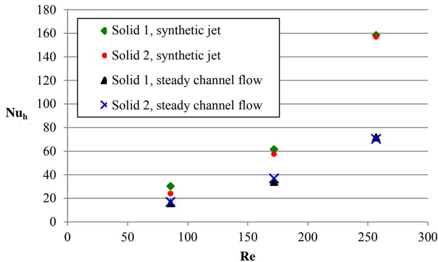
Figure 4.  $Nu_h$  vs.  $Re$  for both Solid configurations and  $1St$  case.
