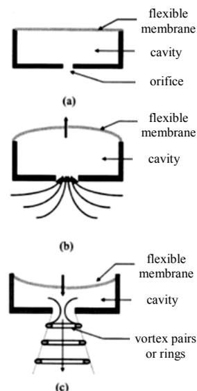
Figure 1. Schematic of a synthetic jet actuator and its operation: (a) basic components; (b) suctioning phase; (c) ejection phase and formation of synthetic jet.
