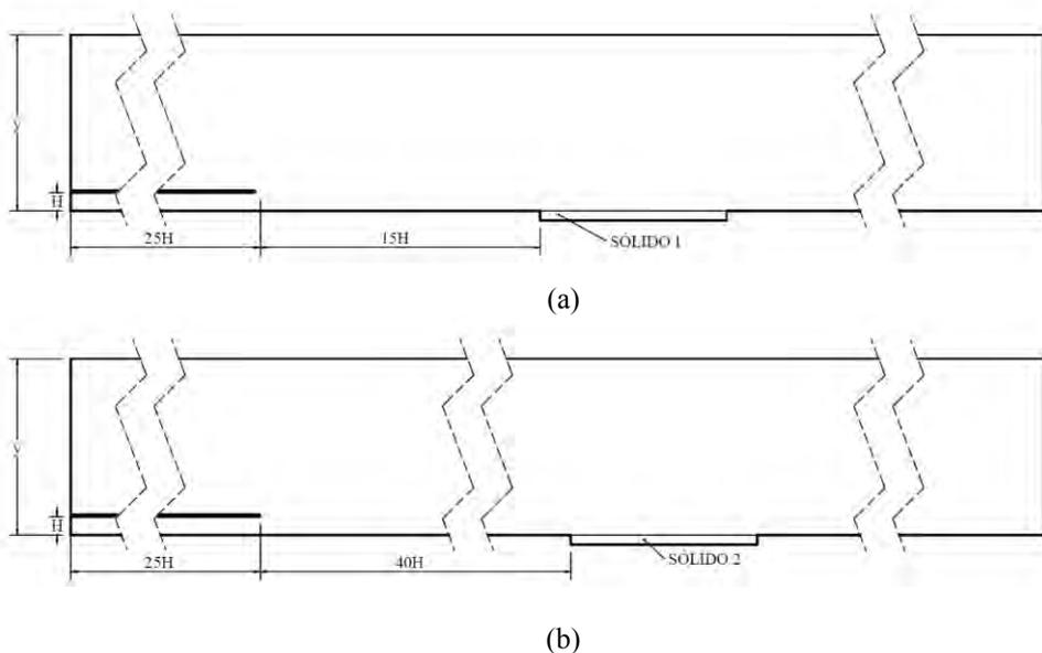
Figure 2. Schematic of channel geometries used in this study: (a) Solid 1 and (b) Solid .
