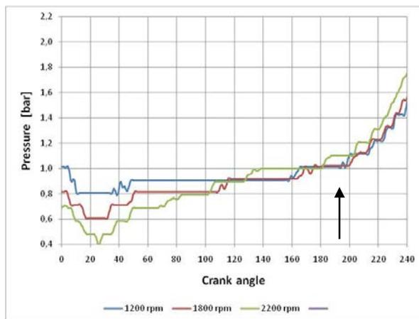
Figure 4. Locating the inlet valve closure
