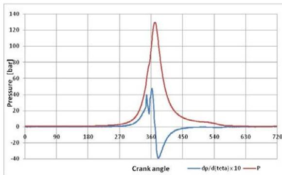
Figure 2. Experimental pressure and pressure derivative as functions of crank angle.
