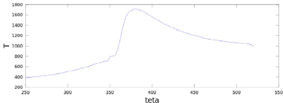
Figure 9. Calculated average temperature from experimental data for 1200 rpm.
