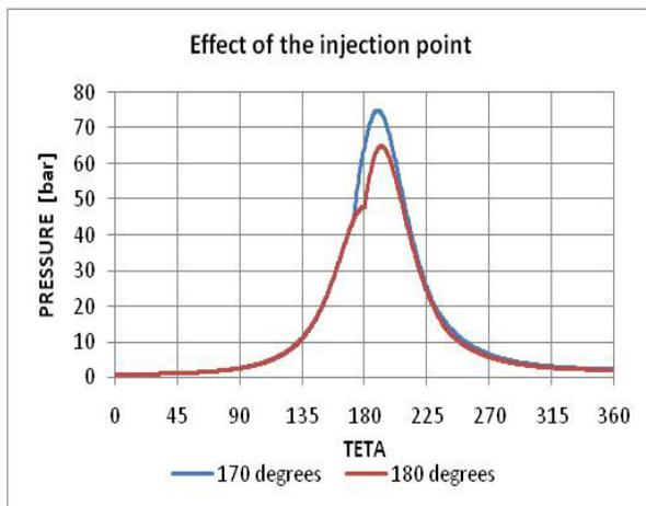
Figure 13. Pressure as a function of crank angle.
