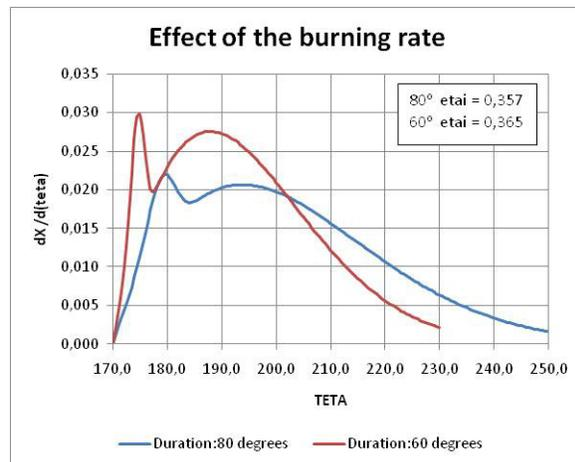
Figure 14. Heat release rates for different combustion. duration: 60° (base) x 80° crank angle
