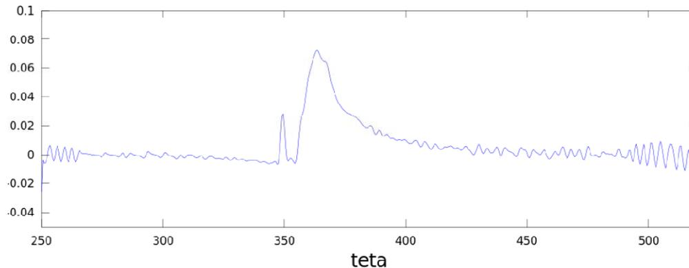
Figure 6. Calculated apparent heat release for 1200 rpm.
