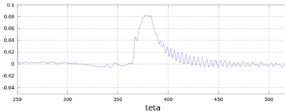
Figure 7. Calculated apparent heat release for 2200 rpm.
