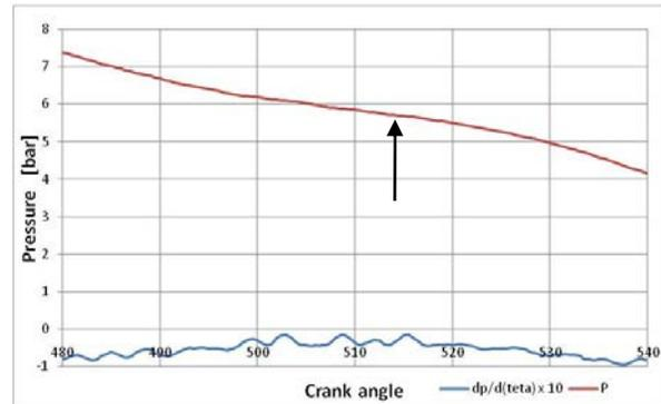
Figure 3. Locating the exhaust valve opening
