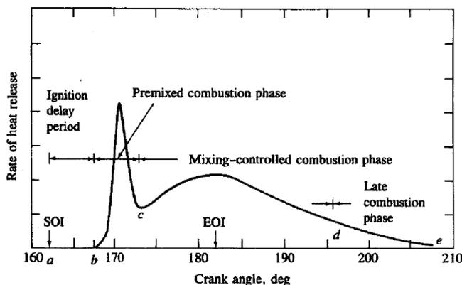
Figure 1. Identification of the phases of the combustion, from heat release rate (Heywood, 1988).
