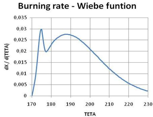
Figure 12. Diesel engine burning rate simulation.
