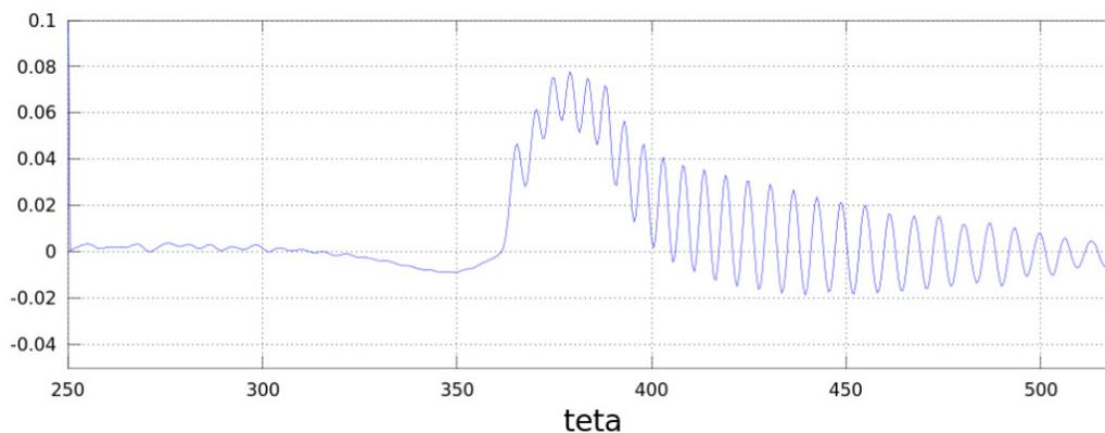
Figure 8. Calculated apparent heat release for 3200 rpm.
