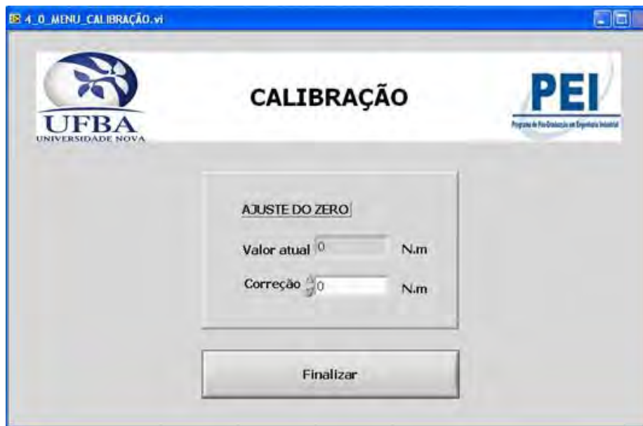
Figure 9. Print screen of the software load cell calibration menu window developed
