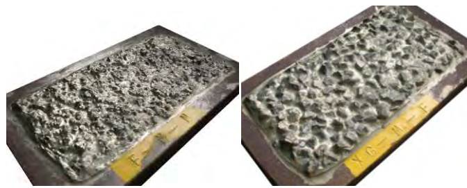
Figure 6. Brazed deposit over test plate (250 x 150 x 25.4 mm) for fine (left) and coarse (right) granulometries
