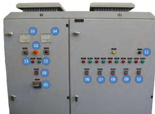
Figure 11. Electric board: 01 – On/Off; 02 – Emergency stop; 03 – Voltage reading; 04 – Current reading; 05 – Rotation motor; 06 – X axis; 07 – Y axis; 08 – Z axis; 09 – Pumping system; 10 – Heating system; 11 to 13 – Automatic mode
