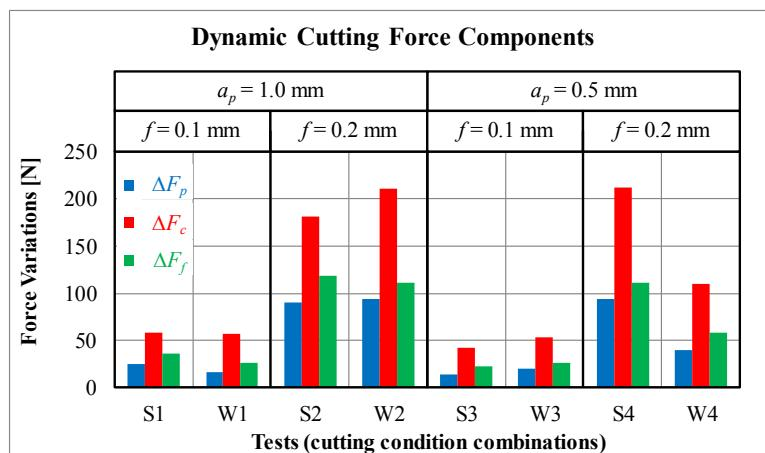
Figure 11. Dynamic cutting forces in turning of AISI 420 (95% of confidence interval).
