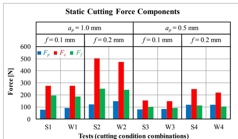
Figure 10. Static cutting forces in turning of AISI 420
