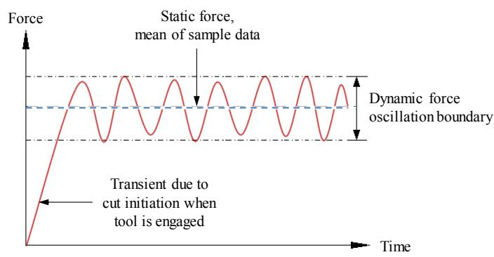
Figure 2. Force amplitude vs. time (fixed cutting conditions) (adapted from Dimla, 2000).
