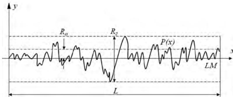
Figure 3. Roughness  $R_a$  e  $R_z$  on a surface profile  $P(x)$  of an evaluation length  $L$  (adapted from Mello *et al.*, 2012)
