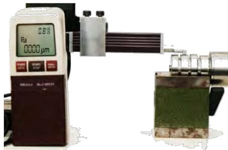
Figure 9. Surface roughness measurement equipment Mitutoyo SJ-201 and workpiece machined
