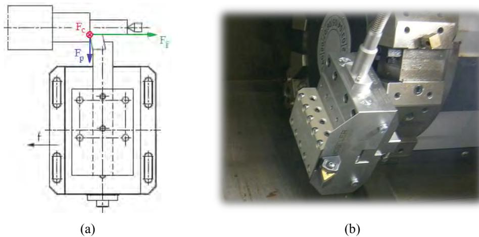
Figure 8. Kistler stationary dynamometer model 9129A: (a) draw of forces during longitudinal cylindrical turning (adapted from Kistler, 2009); (b) 3-component system installed on Mazak QTN 100-II
