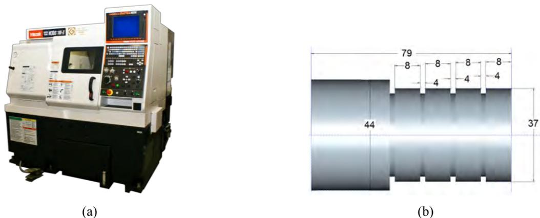
Figure 6. (a) CNC lathe Mazak QTN 100-II; (b) workpiece used in the experiment
