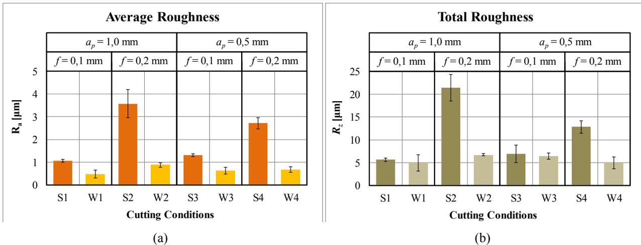
Figure 12. Roughness parameters and its expanded uncertainty with 95% of confidence interval: (a)  $R_a$ , (b)  $R_z$
