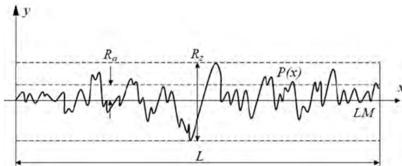
Figure 3. Roughness  $R_a$  e  $R_z$  on a surface profile  $P(x)$  of an evaluation length  $L$  (adapted from Mello *et al.*, 2012)
