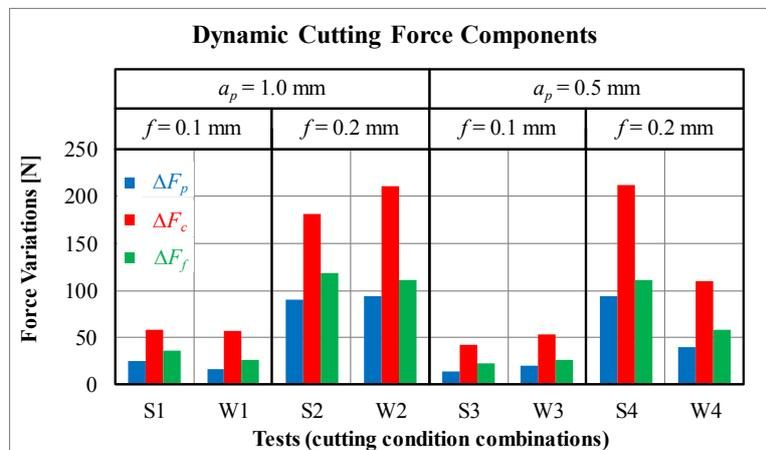
Figure 11. Dynamic cutting forces in turning of AISI 420 (95% of confidence interval).
