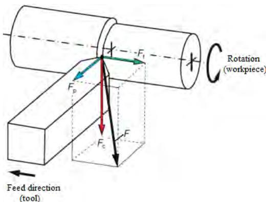
Figure 1. Cutting forces in turning.
