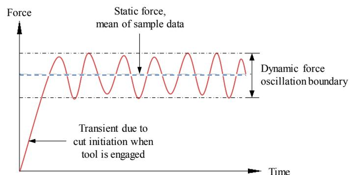
Figure 2. Force amplitude vs. time (fixed cutting conditions) (adapted from Dimla, 2000).
