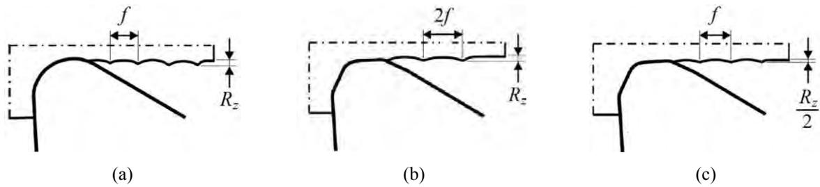
Figure 4. Scheme on surface roughness formation ( $R_z$  parameter) during the turning process: (a) standard geometry and (b-c) wiper geometry (Stachurski *et al.*, 2012)
