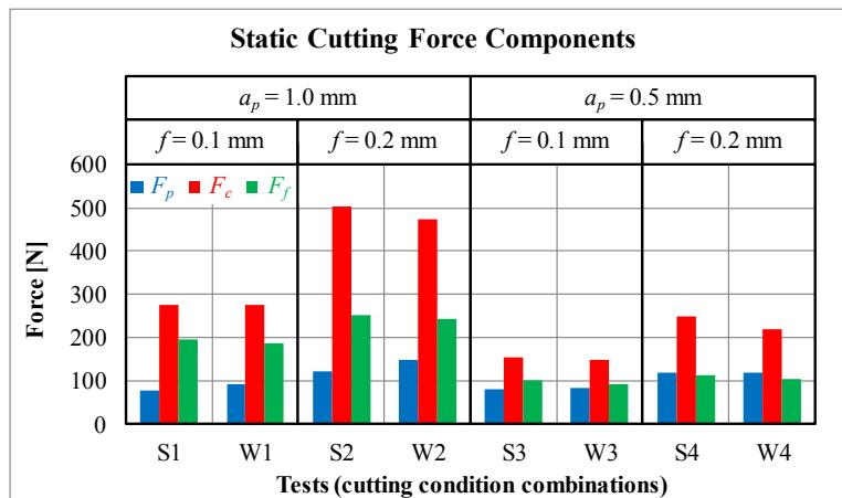
Figure 10. Static cutting forces in turning of AISI 420
