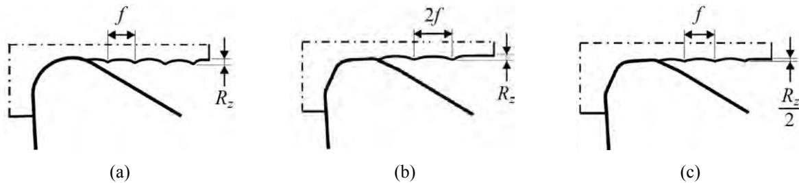
Figure 4. Scheme on surface roughness formation ( $R_z$  parameter) during the turning process: (a) standard geometry and (b-c) wiper geometry (Stachurski *et al.*, 2012)
