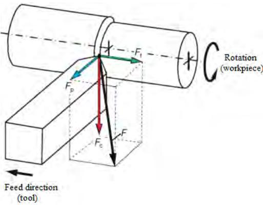
Figure 1. Cutting forces in turning.
