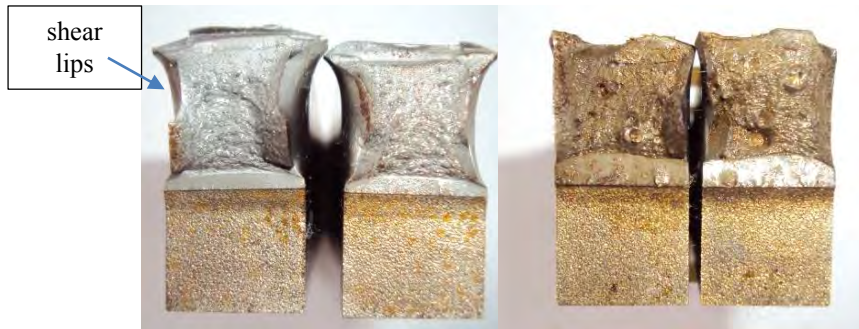
Figure 6: (a) base metal specimen crack surface after CTOD test; (b) weld metal specimen crack surface after CTOD test.
