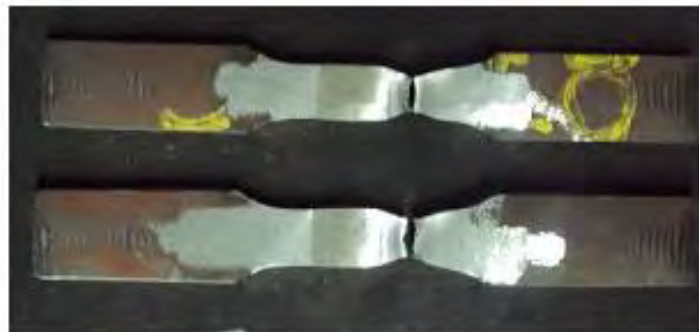
Figure 5: Tensile samples broken at the base metal.
