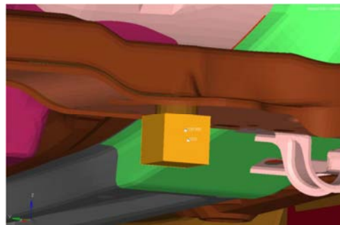
Figure 5 – Finite element model, cradle- suspension zone (Ref. fig. 3).
