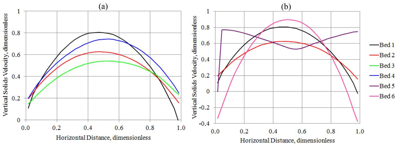
Figure 4. Comparison between the horizontal profiles of vertical velocity. Real, scaled and change in particle diameter (a). Real, scaled and change in superficial gas velocity (b). Elevation of 8.4 m.
