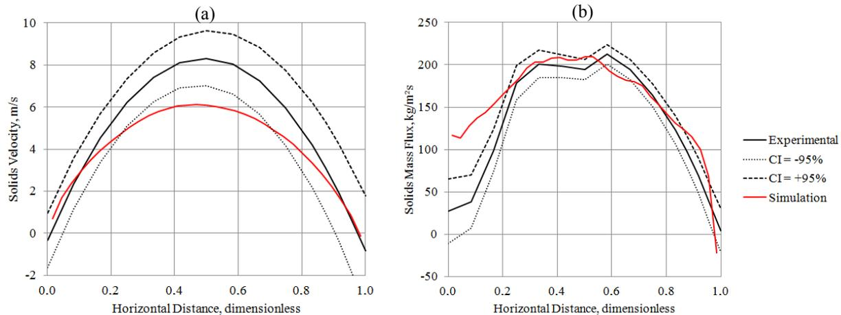
Figure 2. Experimental validation of the numerical model for the full-scale reactor. Horizontal profile of the vertical solids velocity (a) and solids mass flux (b). CI is the confidence interval of 95% for the experimental data. Elevation of 8.88 m in bed.
