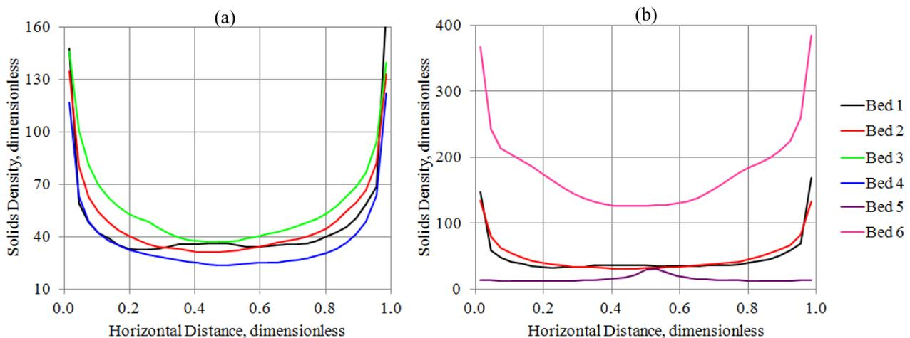
Figure 3. Comparison between the horizontal profiles of solids mass density. Real, scaled and change in particle diameter (a). Real, scaled and change in superficial gas velocity (b). Elevation of 8.4 m.
