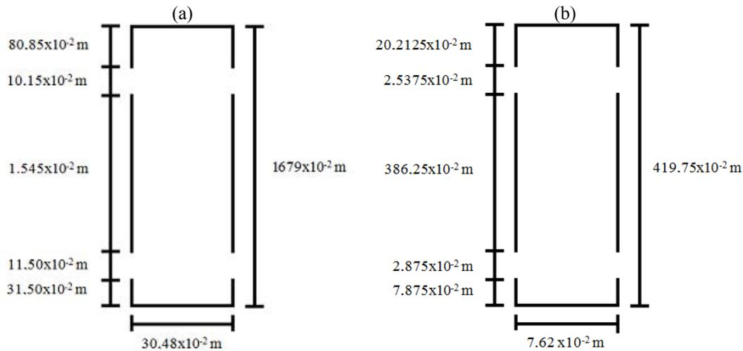
Figure 1. Geometric model used in the simulations for the full-scale bed (a) and scaled bed (b).
