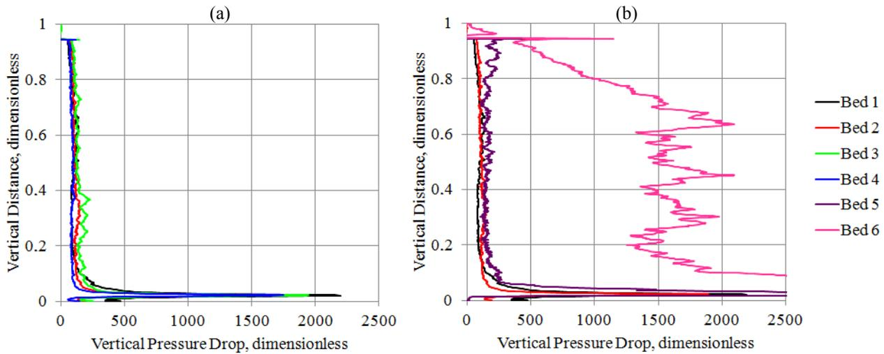
Figure 5. Comparison between vertical profiles of pressure drop between the beds. Real, scaled and change in particle diameter (a). Real, scaled and change superficial gas velocity (b).
