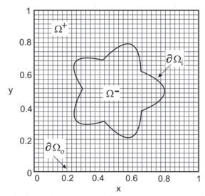
Figure 1. Illustration of the domain for the immersed interface problem, extracted from (Linnick and Fasel, 2005).
