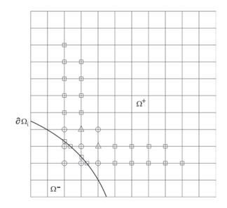
Figure 2. Stencil intersected by the immersed interface, extracted from (Linnick and Fasel, 2005). In the figure, ( $\bigcirc$ ) represents the points of the stencil from (31) and ( $\Box$ ) the correction terms. The points where ( $\bigcirc$ ) and ( $\Box$ ) overlap are represented by ( $\triangle$ ).
