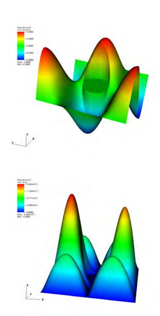
Figure 3. Solution for the Poisson equation (40) using the IIM-I. On the top, the numerical solution, and below, the corresponding error for a  $400 \times 400$  grid.
