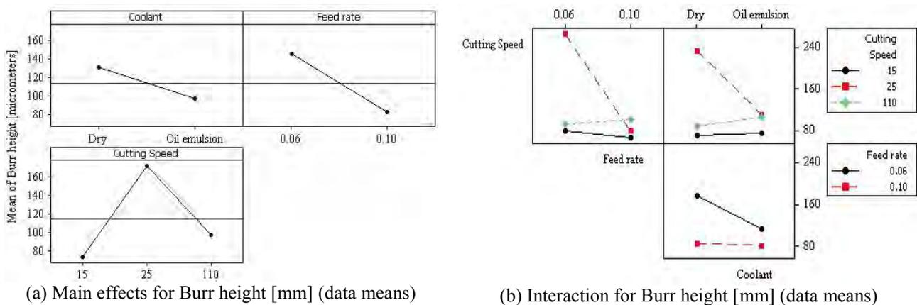
Figure 7. Graph of main effects and interaction for Burr height
