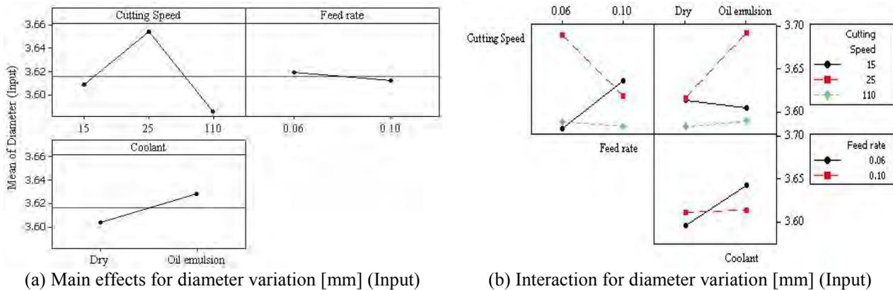
Figure 8. Graph of main effects and interaction for input diameter
