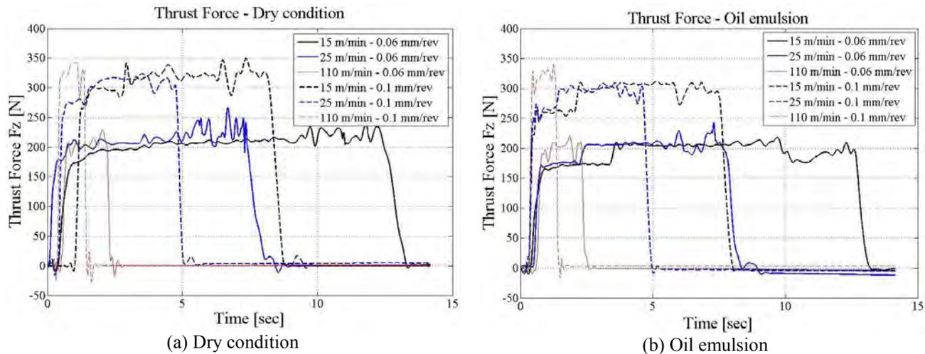
Figure 2. Thrust Force Fz all trials in dry condition and oil emulsion
