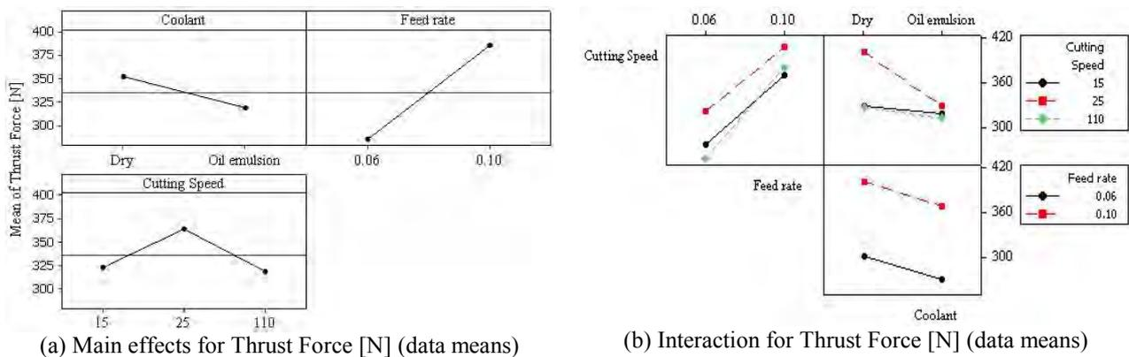
Figure 3. Graph of main effects of Thrust Force
