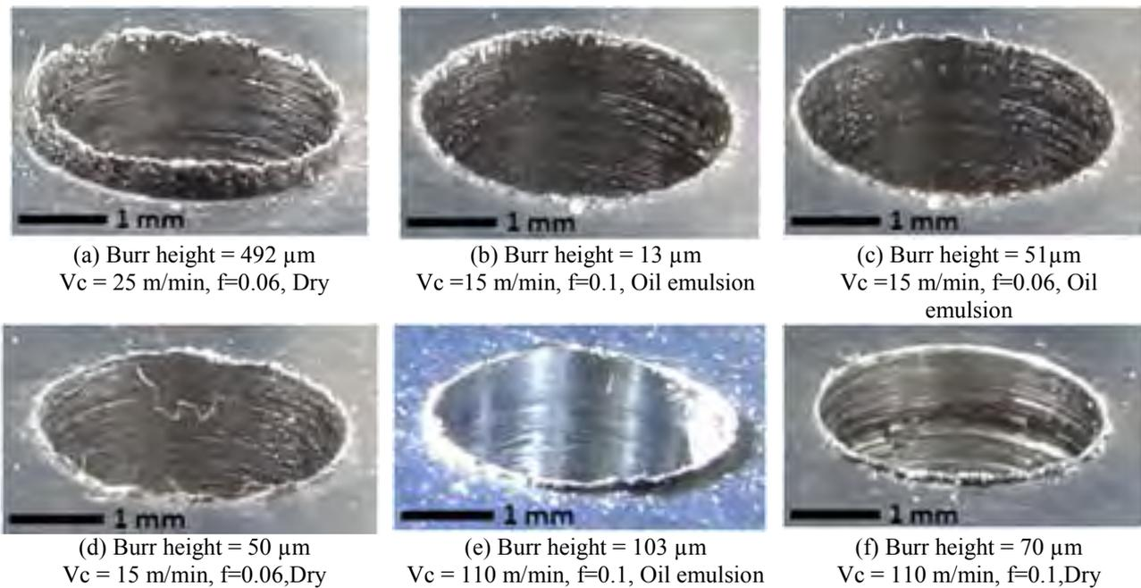
Figure 6. Burrs used in the set-up of drilling
