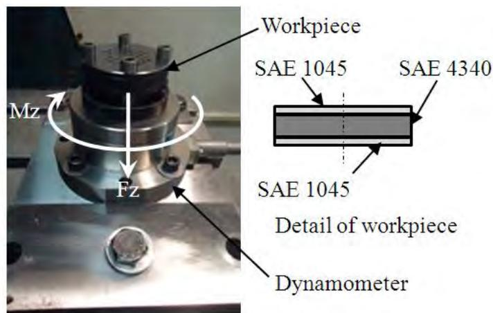
Figure 1. Set-up of experiments to measure Thrust Force and Torque and scheme of bimetallic work piece used in experimental tests
