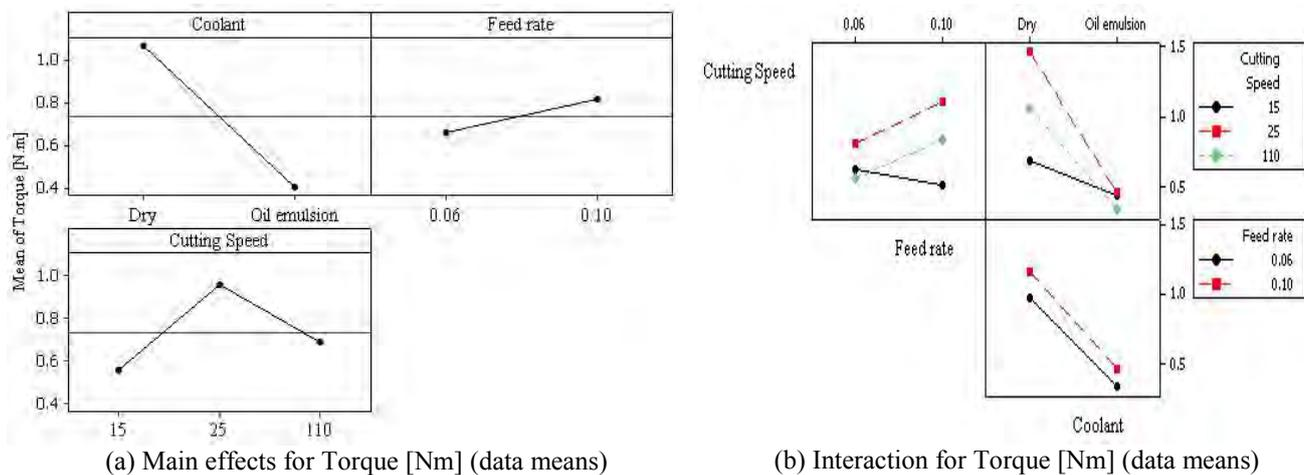
Figure 5. Graph of main effects and interaction for Torque
