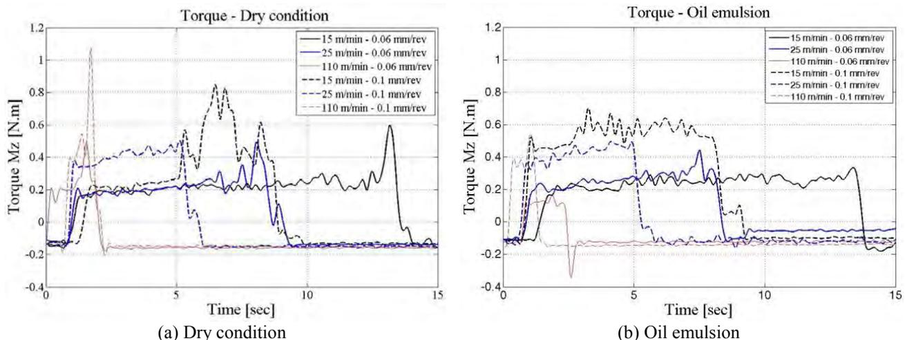
Figure 4. Torque Mz for all trials in dry condition and oil emulsion
