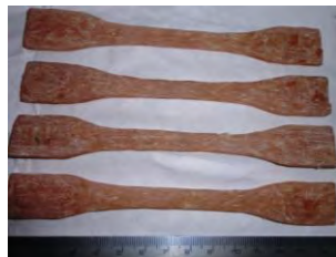
Figure 3. Sisal/Glass hybrid composites.
