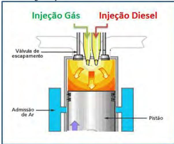
Fig. 1. Arrangement of pilot diesel injection and gas injection in the combustion chamber [4].
