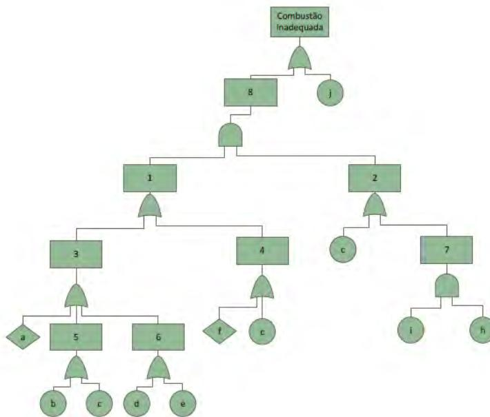
Fig 4. Construction of the Diesel Gas Kit Fault Tree for inadequate combustion<sup>[4]</sup>.
