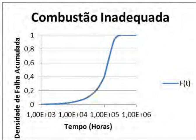
Figure 7. Failure Estimate versus Diesel Gas Kit Time for Inadequate Combustion
