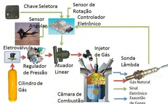
Fig. 2. Third generation Diesel Gas Kit operating diagram [4].
