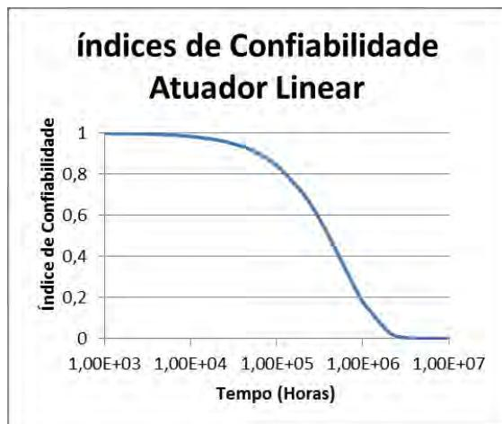
Fig. 6. Graph: Reliability versus Linear Actuator Time [4].
