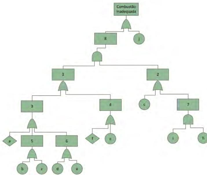
Fig 4. Construction of the Diesel Gas Kit Fault Tree for inadequate combustion [4].
