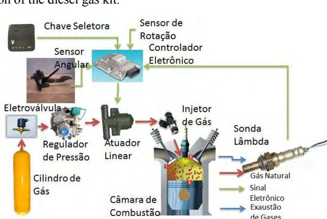
Fig. 2. Third generation Diesel Gas Kit operating diagram [4].
