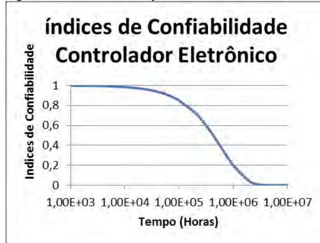
Fig. 5. Graph: Reliability versus Electronic Controller Time <sup>[4]</sup>.
