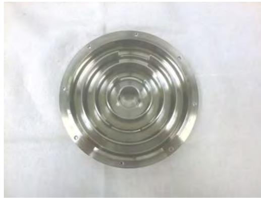
Figure 2 – View of the internal part of the humidity generator
