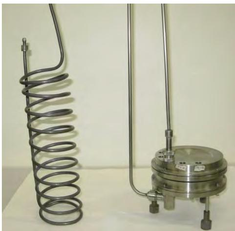
Figure 1 – Pre-saturator (L) and saturator (R)
