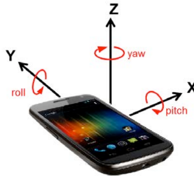
Figure 10. Definition of degrees of movement in three-dimensional space.
